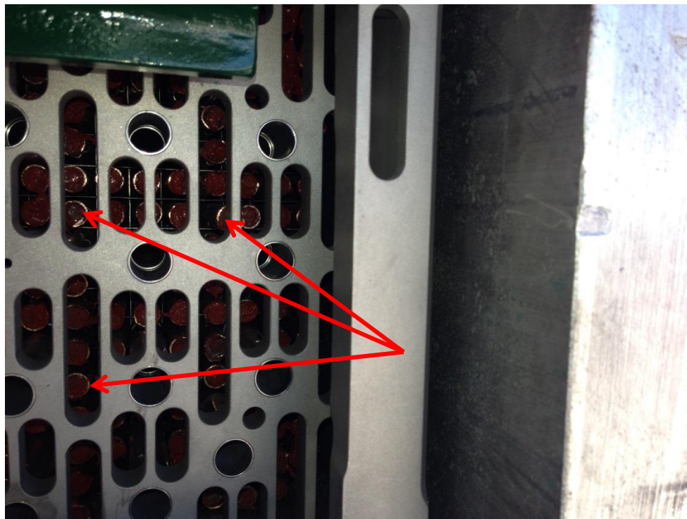
Figure 3.3 The red arrows point to some of the copper rods that moved longitudinally within the assembly during the truck test.
