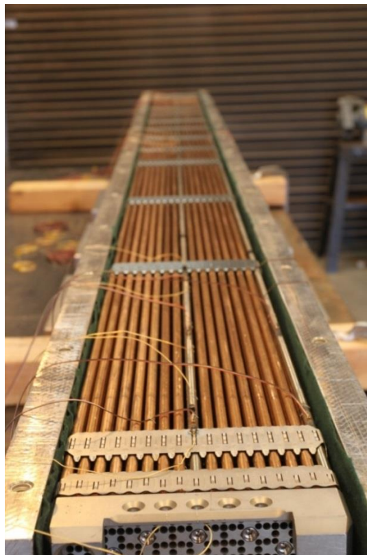
Figure 3.6 Assembly in basket with top plate of basket removed (side plates are visible). This figure shows two Zircaloy-4 rods (center and right edge). Only the center Zircaloy-4 rod was used for the truck test.
