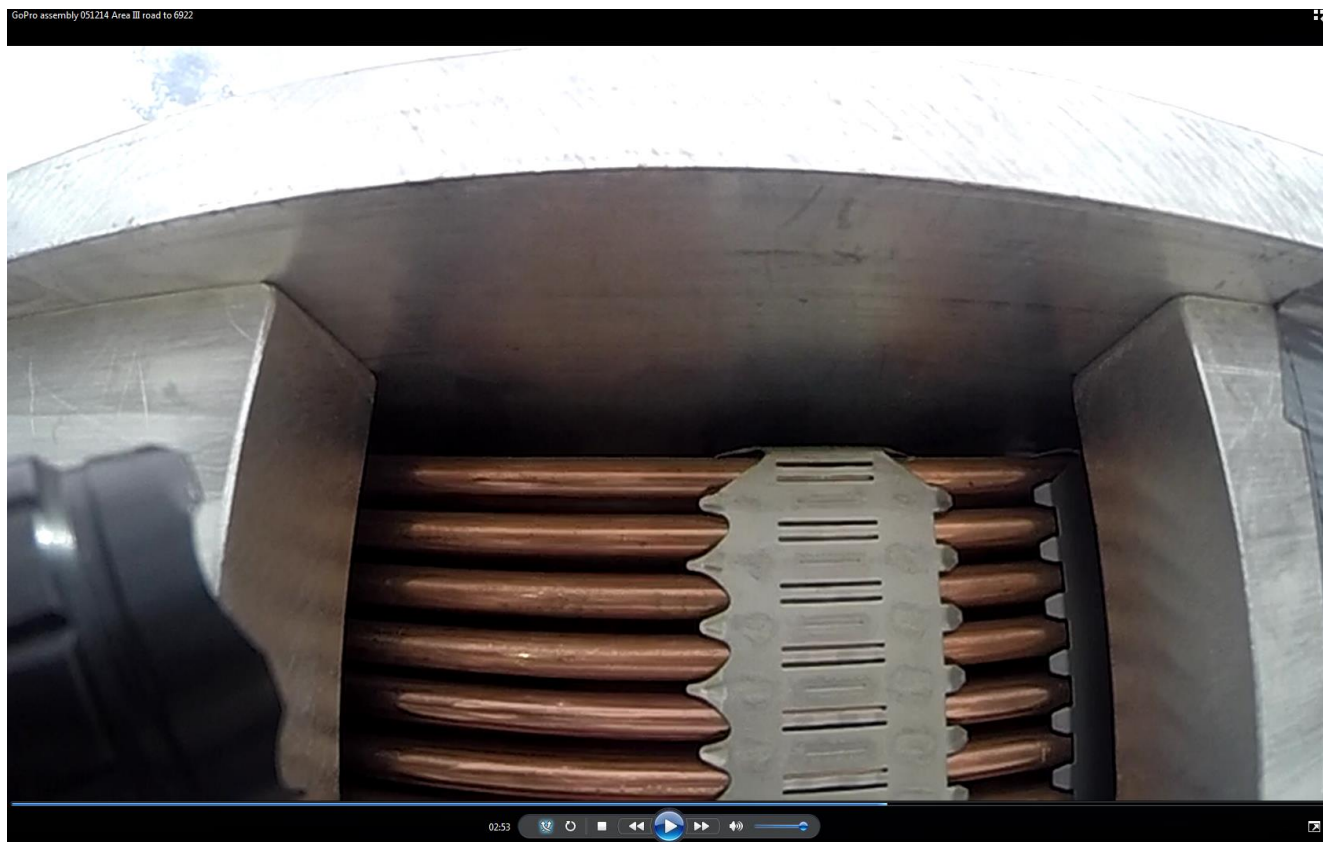
Figure 5.3 Screen capture of GoPro® .MP4 video file. There was no observed motion of the assembly relative to the inside of the top basket plate or the copper rods relative to one another or relative to the spacer grid in the 4 minute 23 second video (240 frames/second). There was occasionally motion observed between the top edge of the top basket plate relative to the clouds in the sky (note bluish-gray patch in top left corner of figure). The perceived curvature is an artifact of the wide angle view of the video.
