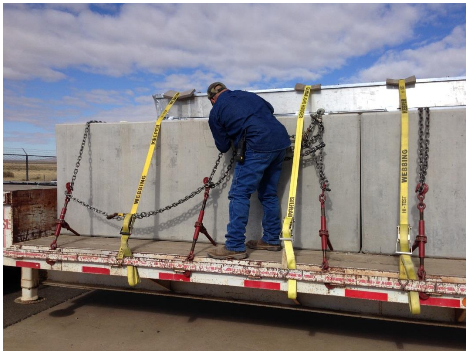
Figure 3.15 Concrete blocks simulating the mass of a truck cask were secured to the trailer. The basket was bolted to the blocks (Figure 3.16).
