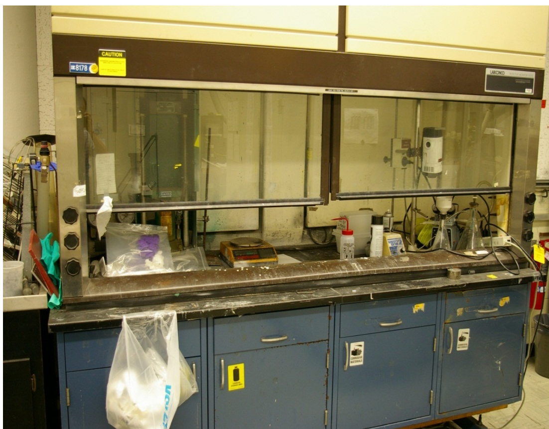
Figure 3-4. Fume Hood Used for Sample Etching with Hydrofluoric (HF) and Nitric (HNO 3 ) Acids.
