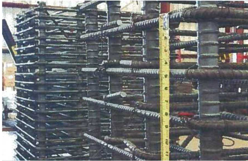
Figure 3. Reduction in rebar density with the use of high-strength rebar (conventional 60 ksi rebar [left] versus 100 ksi high-strength rebar [right])
