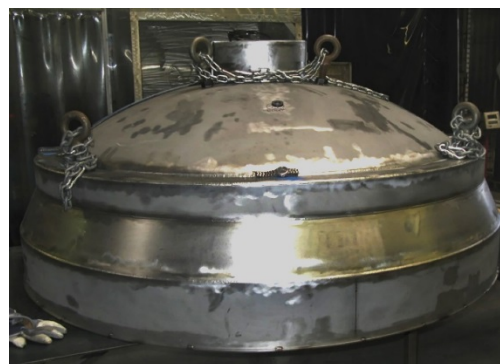
A 70-inch (1780mm) one-half diameter capsule (can) was produced in 2017 for the 2/3rds scale lower reactor head, which is to be filled with powder and HIP'ed in 2018.
