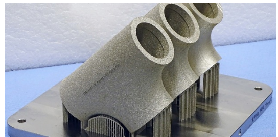
Three 316L stainless steel tee-shaped pipe sections were produced with structural defects implanted into them for characterization.
