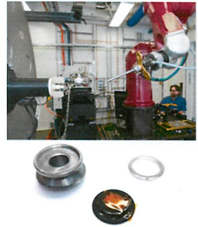
Figure 1 (a) The robot installed at XPD. (b) Radioactive sample holder with magnetic closure ring for rapid loading
