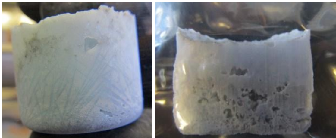
Figure 7-2. Photographs of Surrogate Electrorefiner Salt After Melting and Freezing in the Zone Freezing Furnace.
