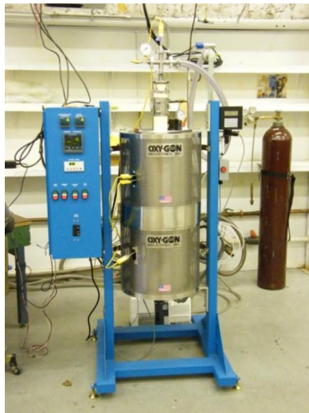
Figure 7-1. Photograph of the Zone Freezing Furnace used for Preparing Surrogate Electrorefiner Salt Samples for Microscopic Evaluation
