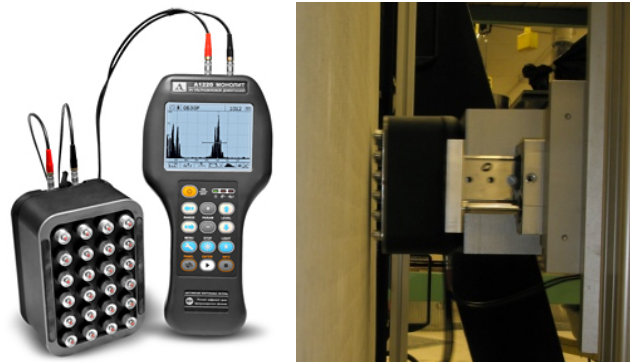
Figure 6. Ultrasonic Sensor. Dry-coupled sensor with at center frequency of 55 kHz, designed for measurements on concrete. Left: Probe with handheld controller. Right: Probe mounted on scanning system for automated use.
