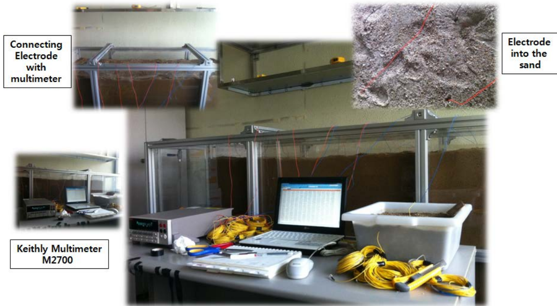
Figure 6.3-3 Full setup of a sandbox experiment (Wang et al. 2015; 2016)
