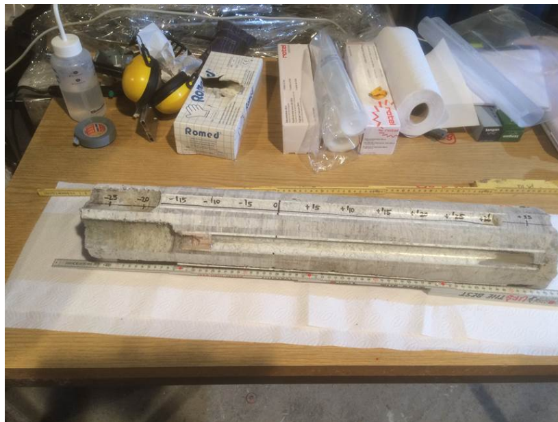
Figure 3.3-11 An overcore that preserves the interface between shotcrete and bentonite (Zheng et al., 2016).
