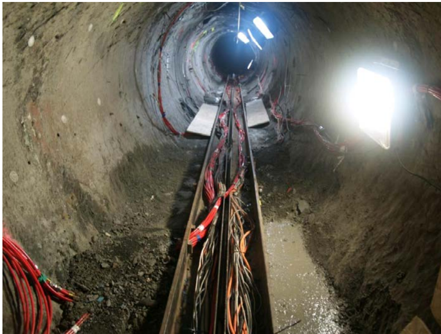
Figure 3.1-10 HE-E Heater Test at Mont Terri URL: Photo of micro-tunnel before buffer emplacement.
