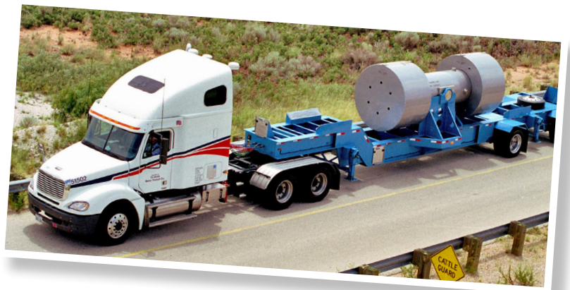
Cask in transport for disposal at the Waste Isolation Pilot Plant, a deep geologic repository for transuranic waste (not spent nuclear fuel or high-level radioactive waste) near Carlsbad, New Mexico.
