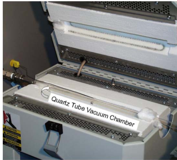
(b) Quartz Tube Inside Furnace
