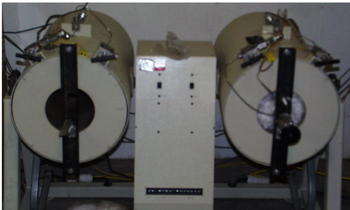
Figure 2.3. 400°C/600 bar rocking autoclave rack (autoclave drums are ~24" tall)
