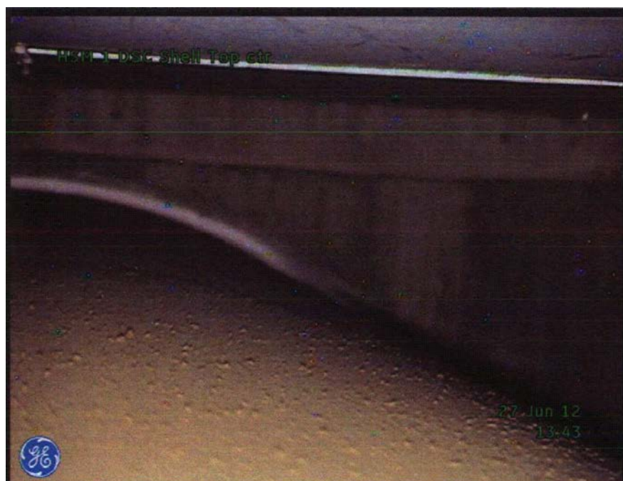
Figure 4. Photograph of dust on the surface of the waste container, Calvert Cliffs container inspection, June, 2012.
