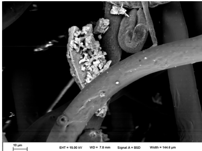
Figure 12. SEM BSD photo, EDS spectrum, and element maps of EPRI filter #1, showing close-up of the multicomponent mineral grain in Figure 9D (Note that pattern of fiber is beam damage).
