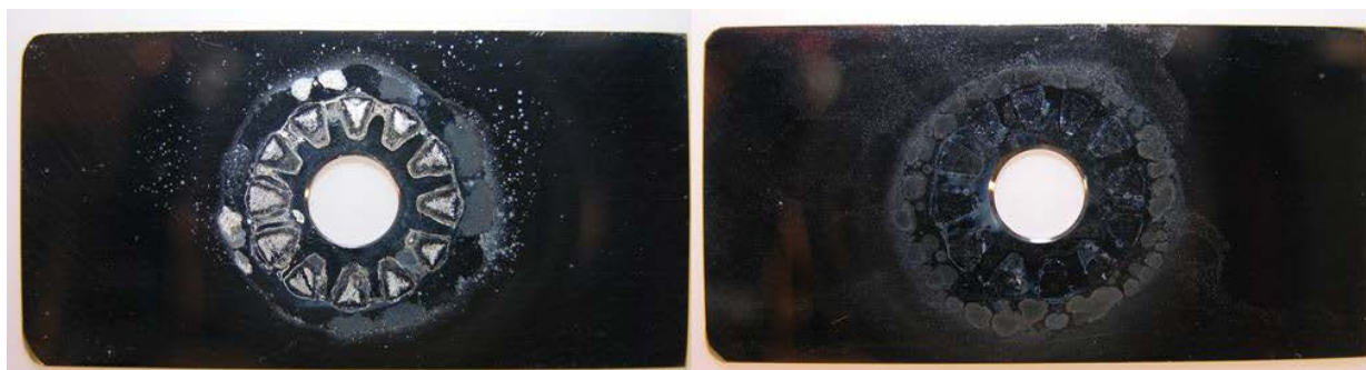
Figure 8. 304SS coupon with 200 \mu\text{g}/\text{cm}^2 and 7 day exposure after crevice former removal (L) and rinsing (R).
