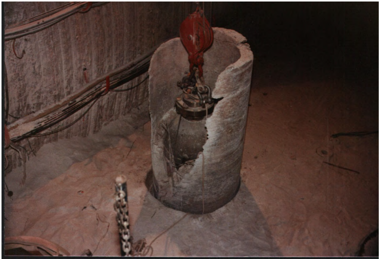
Figure 52: Heater from borehole BO45 showing porosity reduction as a likely result of heat pipe activity (Krumhansl et al., 1991). From Brady et al. (2013).
