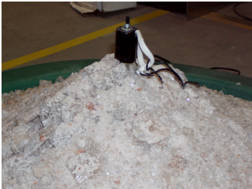
Figure 25: Crushed salt cone experiment with a 125W light bulb at the apex of the cone.
