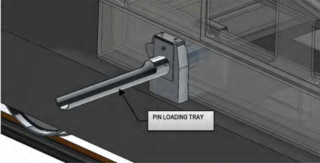
**FIGURE C-16: PIN LOADING TRAY WITH PIN RETRACTED**
