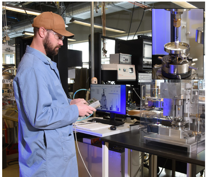
Figure 1. Defueling module removing first pellet from one end of a prototype fuel rod.
