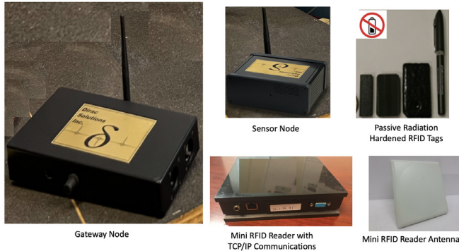
Figure 2: Components of WISLO system uses sensor network nodes and passive RFID through-wall communication transceivers.
