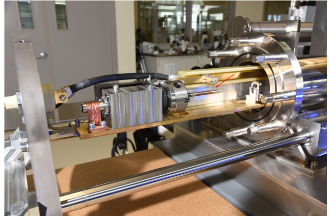
Figure 3. Prototype fuel rod installed in welding chamber with tungsten electrode positioned for welding
