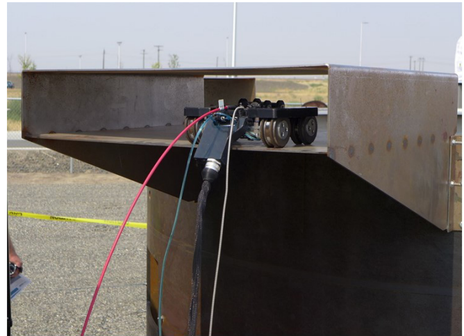
Figure 6. LUS probe being mechanically tested inside a DCSS mockup. Left: entering access vent. Right: inside vertical 2” annular space between canister and concrete overpack wall.
