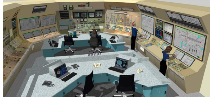
Figure 1. Optimized control board layout with new digital human system interfaces.
