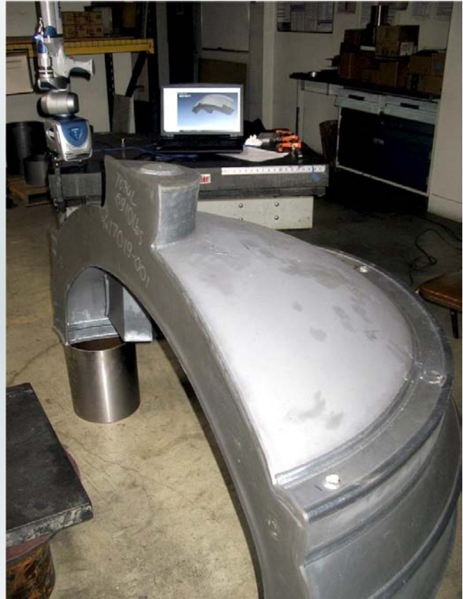
Figure 2. A 2/3-scale, one-half diameter lower reactor head (~70 in. (1780 mm) in diameter, 6910 lbs (3135 kgs) was also produced via PM-HIP.
