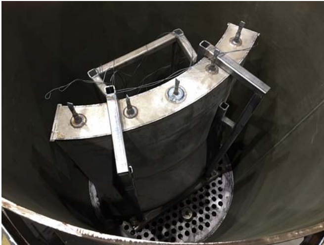
Figure 3. A one-fifth diameter RPV transition shell shown inside of the HIP vessel (with support frame) just prior to HIP'ing.
