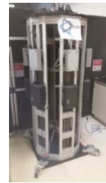
Double Delta system for stress, strain, and radial deformation measurements.
