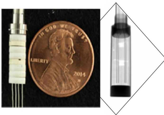
HT MPFD under construction (left) and completed X-ray (right).
