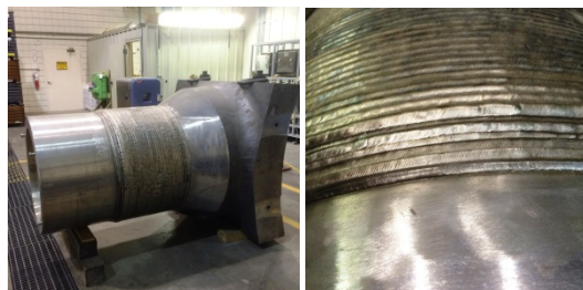
Figure 1. Cladding as butter layer and overlay in DM weld of cold leg to RPV nozzle
