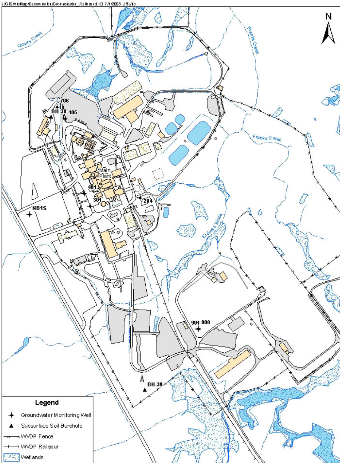
Figure B-3. Onsite Groundwater Wells and Subsurface Soil Boreholes Used as Background
