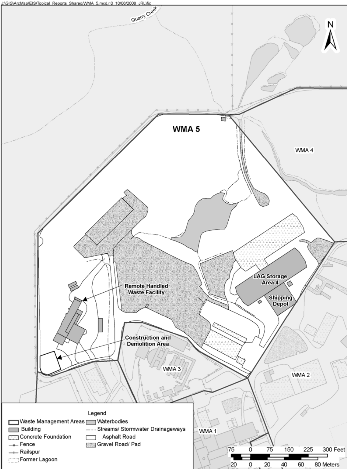
Figure 3-35. WMA 5. (Facilities to be removed during Phase 1 of the decommissioning include the Remote-Handled Waste Facility, Lag Storage Addition 4 and its Shipping Depot.)
