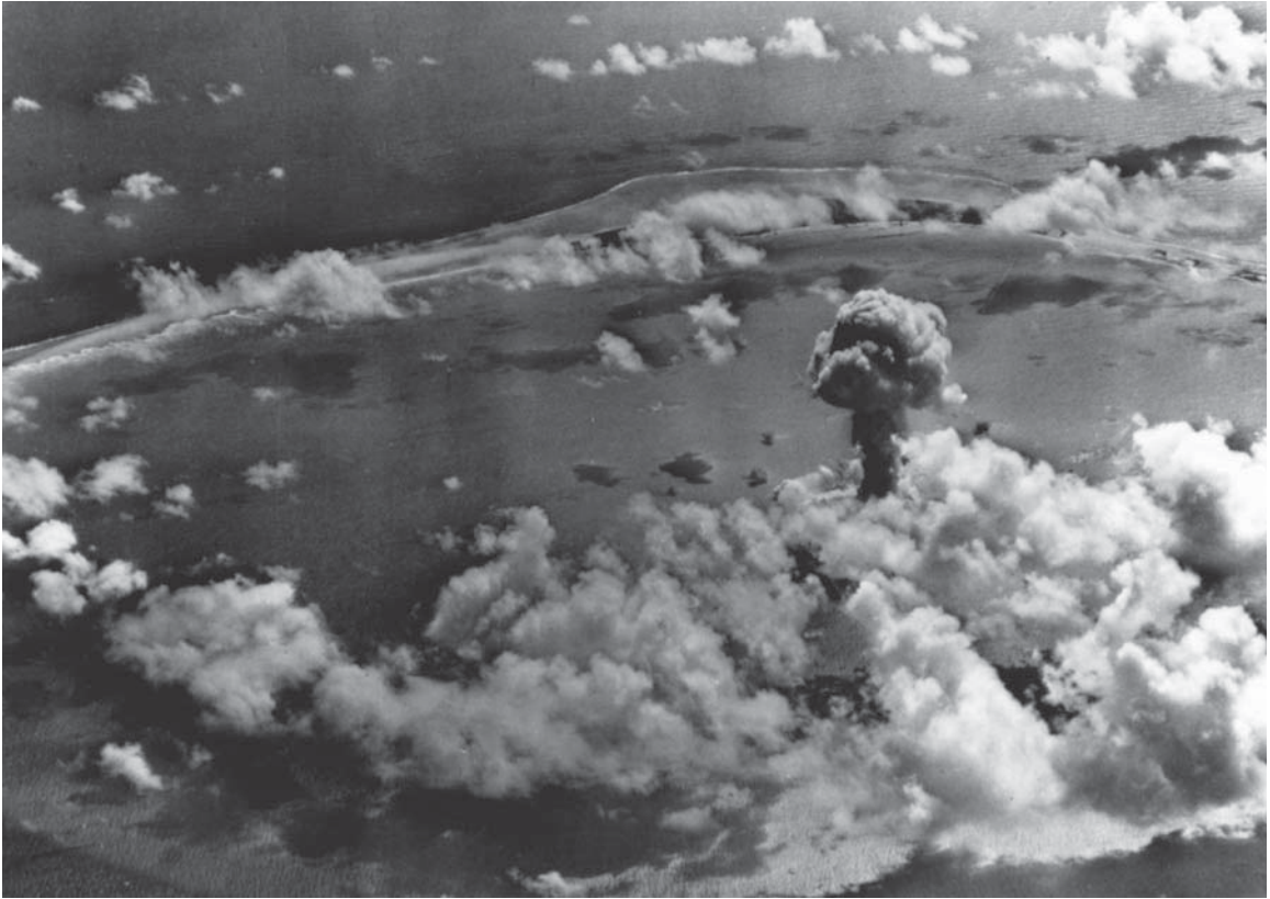
Able test of the Crossroads series, July 1, 1946. Note the shock wave sweeping out around the lagoon. Source: Department of Energy.
