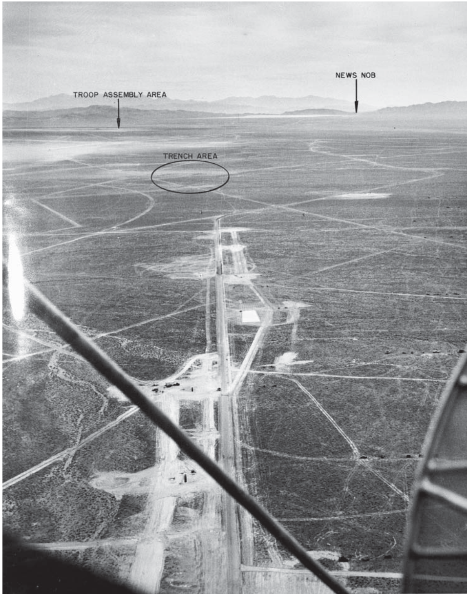
View from the cab of the 700-foot Smoky tower looking south. The tower, momentarily the tallest structure in Nevada, was equivalent in height to a 70-story building. In left foreground are shelters to be tested for the French and German governments. On right side of the photo are military vehicles, part of a blast effects experiment, at varying distances from the tower. The trench area from which military observers will view the test is 4,500 yards from the tower. The troop assembly area is 9,800 yards away, and News Nob is approximately 17 miles distant. Source: DOE, NNSA-Nevada Site Office.
