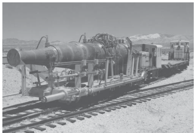
Nuclear ramjet engine on its test bed facility, a railroad flatcar. Source: DOE, NNSA-Nevada Site Office.
