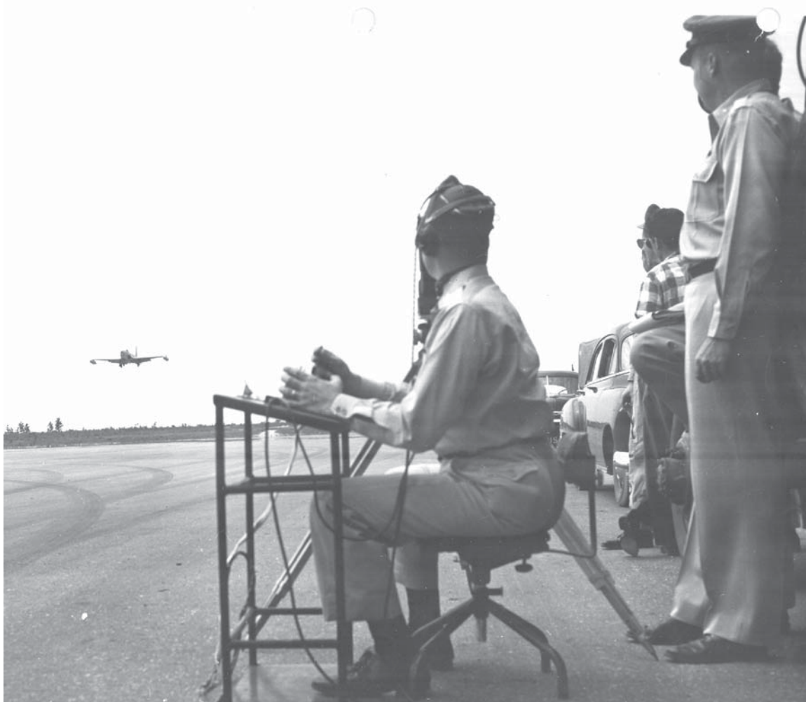
Pilotless QF-80 jet fighter, top, of the Air Proving Ground Command's 3205th Drone Group used to fly through atomic clouds during Operation Teapot. Instrumentation pods slung under the wings, inboard of the fuel tanks, record effects on the aircraft. The drone aircraft, bottom, is being guided in for a landing by its ground controller. Source: DOE, NNSA-Nevada Site Office.
