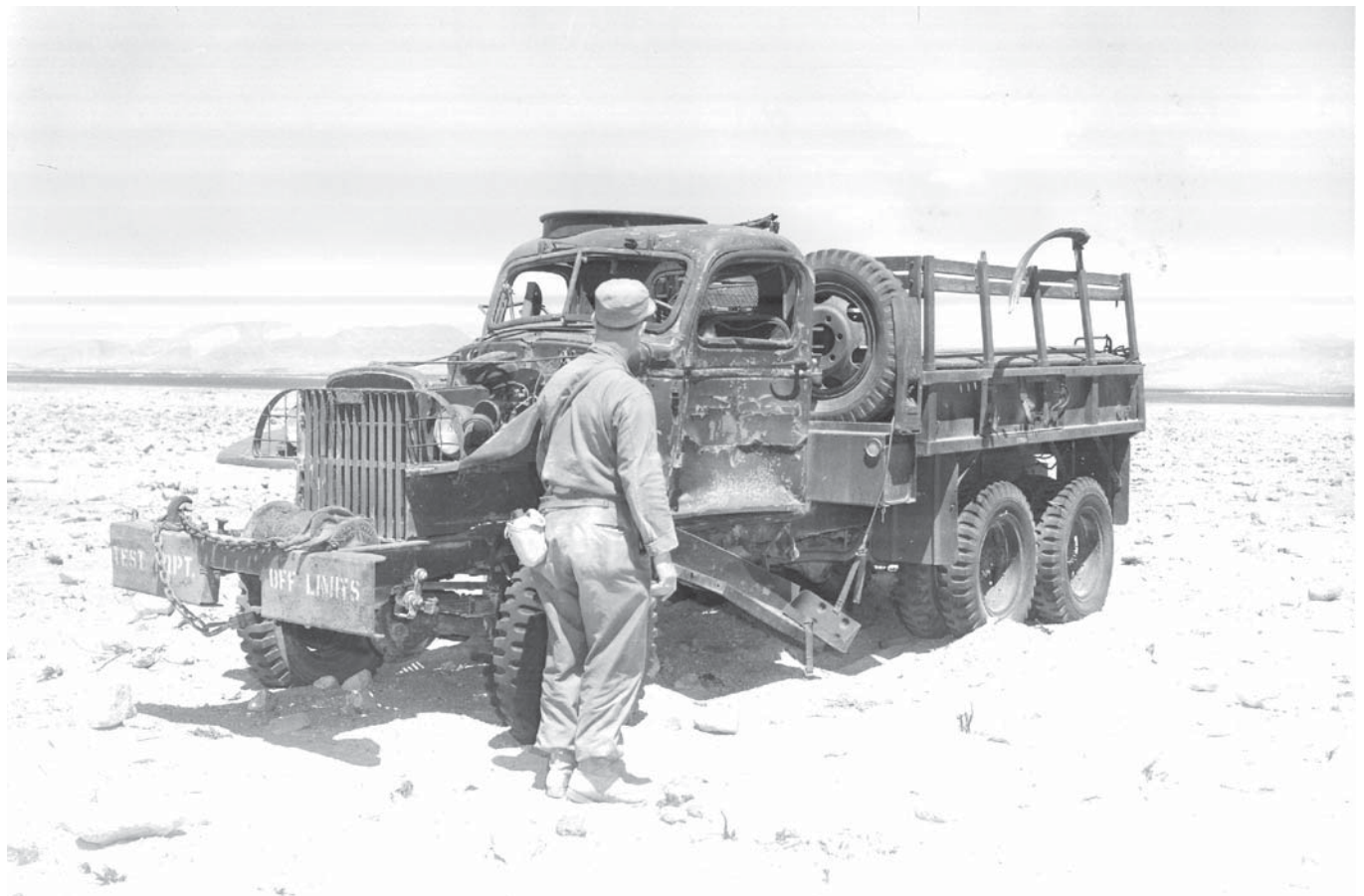
Truck between 400 and 500 yards from ground zero. Source: DOE, NNSA-Nevada Site Office.
