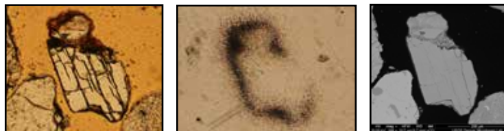
Left to right: Microscope image of a thin section in plain light. Fission-track image of the same grain, where dark "etched" lines are created by uranium decay. Image from the SEM at the U.S. Geological Survey Denver Microbeam Lab, where the circle is the location of elemental analyses, which indicated an iron oxide and clay coating was retaining the uranium seen in the fission-track image.
