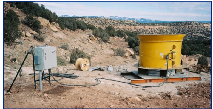
Ventilation fans, such as this one at the C-SM-18 Mine, supply fresh air to the mine workings.
