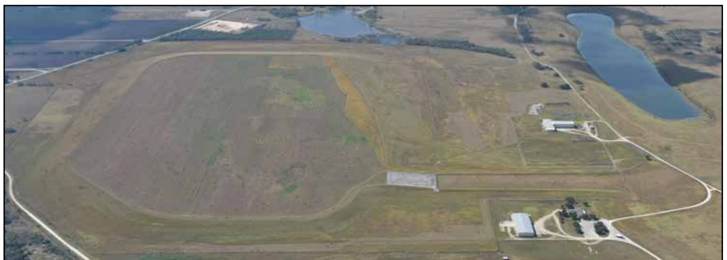
Panna Maria, Texas, Disposal Site. Approximately 6.8 million tons of uranium ore were processed at the former mill, which shut down in 1992. Site reclamation was completed in 2015. The site is expected to transfer to LM for long-term surveillance and maintenance in 2020.
