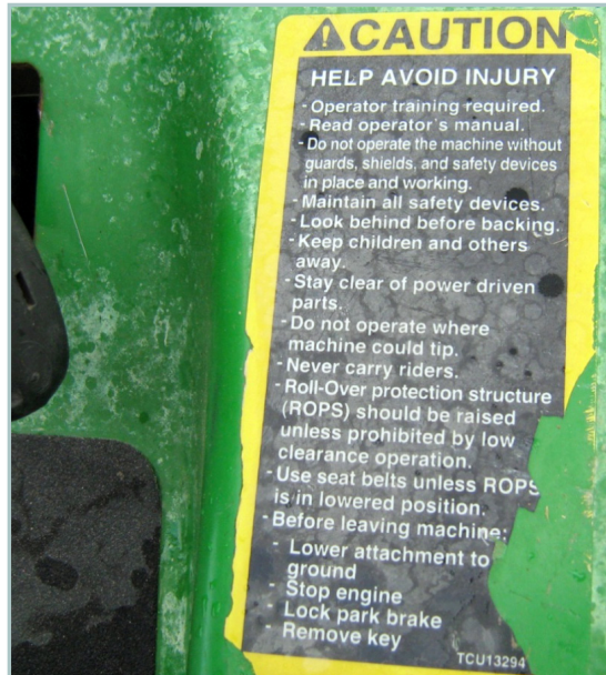
Figure 2-2. Mower-1 warning label facing driver
