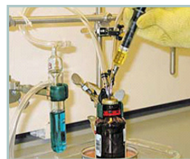
Figure 1-3. Typical setup for syringing t-BuLi
