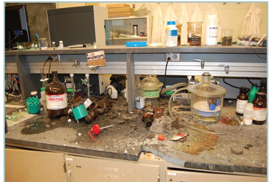
Figure 1-1. Post-explosion view of laboratory table at Texas Tech
