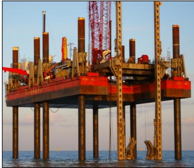
Figure 3-7: Piling Frame on Excilibur Awaiting a Floating Monopile
