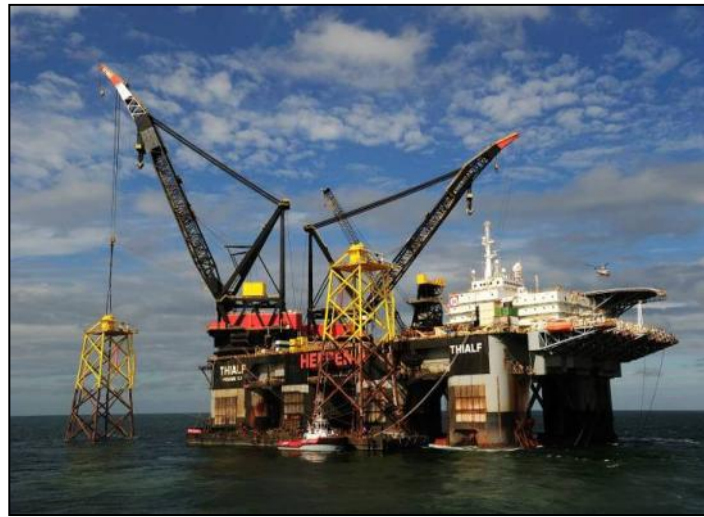
Figure 4-3: Semi-Submersible Heavy Lift Vessel – Jacket installation, by Thialf
