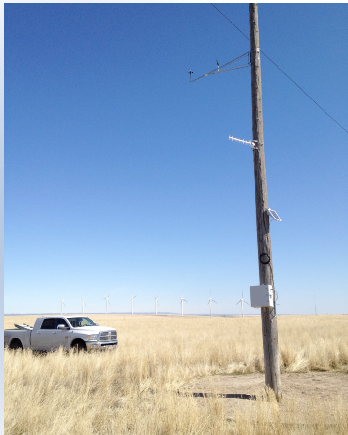
INL researchers and Idaho Power installed 17 weather stations along transmission lines in a windy part of southern Idaho's interstate utility corridor.
