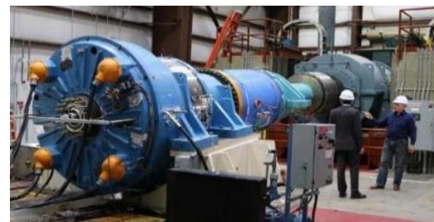
Testing Advanced 750-kW Drivetrain Prototype on 2.5 MW Dynamometer
