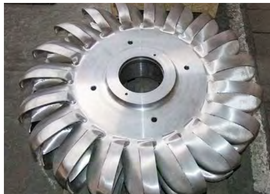
Figure 2-36. Examples of Francis, Pelton, and Kaplan turbines
