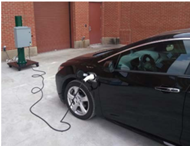
Figure I.20-1 Prototype charging station in action in a test facility on the UNC Charlotte campus.
