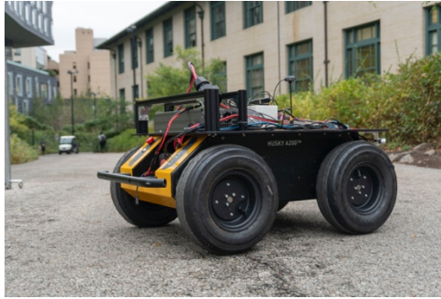
Figure I.12-3 Automated ground delivery robot used for testing (Photo: CMU Team)
