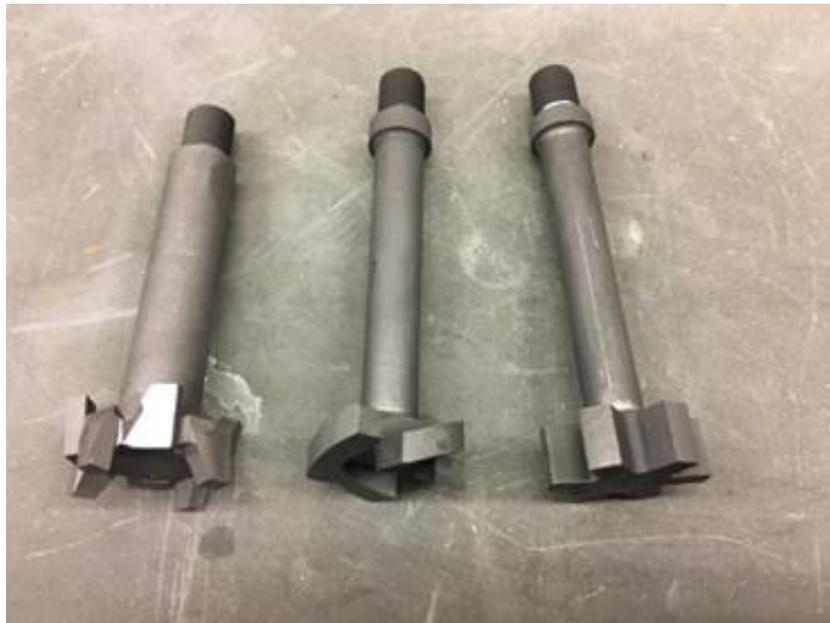
Figure I.2.2.3. Impeller designs for mixing trials. Source: PNNL.
