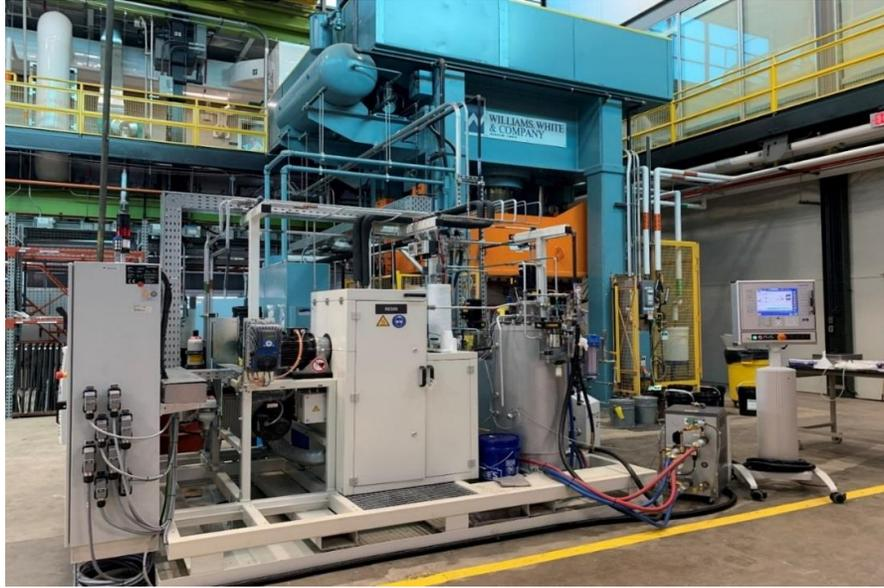
Figure II.2.5.10. HP-RTM metering system installed at GM R&D for the project. Source: GM.
