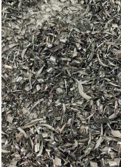
Figure I.3.5.3.2. AA7075 machined chips as feedstock material. Source: ORNL.
