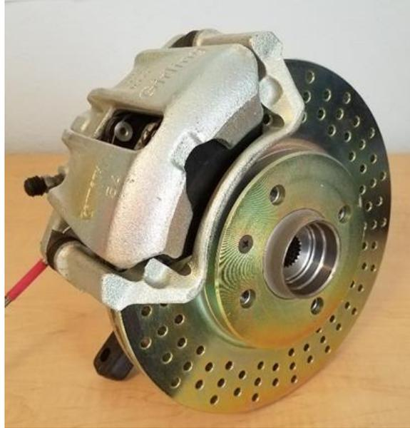
Figure I.2.2.1. Conventional Brake design utilizing an Al caliper and a cast-iron brake disc. Source: PNNL.
