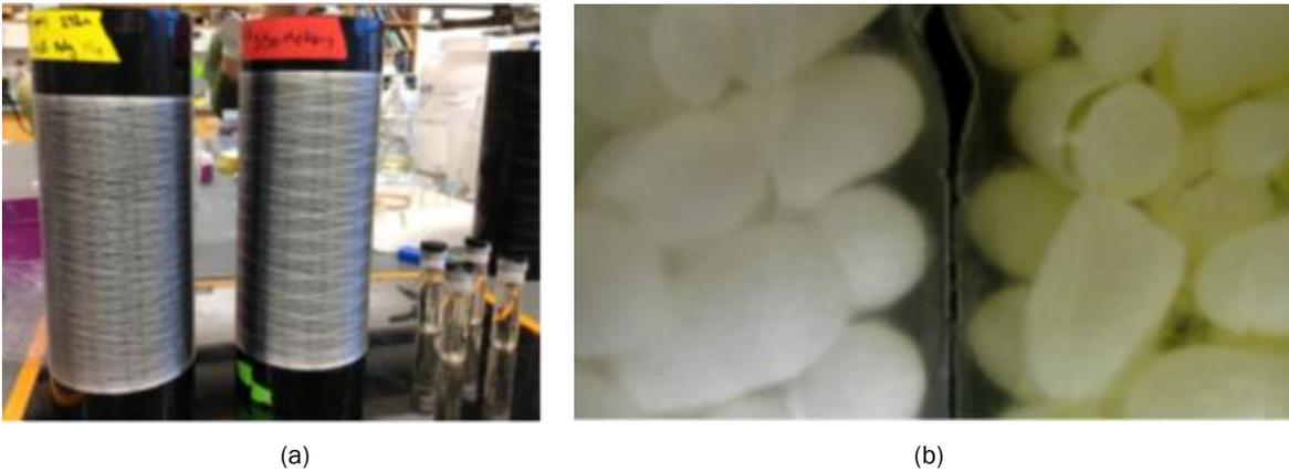
Figure II.2.9.1. (a) Spooled samples of 100% bacterially produced spider silk fiber; and (b) comparative photos of the natural (white) and transgenic silkworm silk (green). Source: USU.
