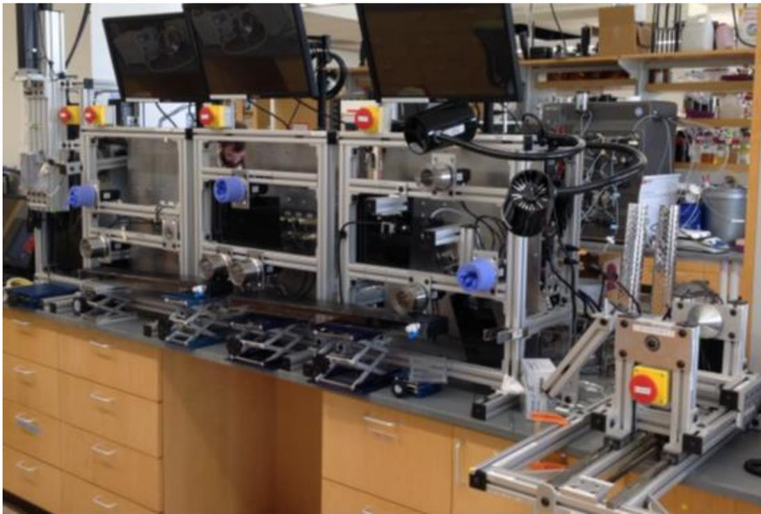
Figure II.2.9.2. Spinning equipment used at USU for the filament extrusion. Source: USU.
