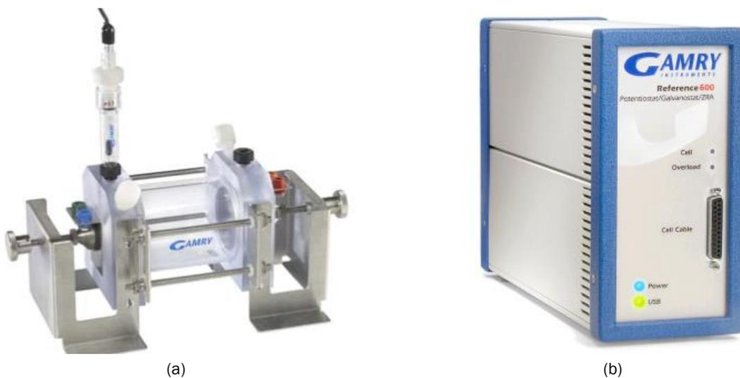
Figure II.3.2.7. (a) Gamry paracell kit; and (b) Reference 600 potentiostat. Source: Gamry Instruments.
