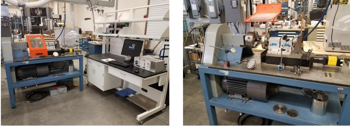
Figure I.2.2.4. Brake friction pair test stand at PNNL. Source: PNNL.
