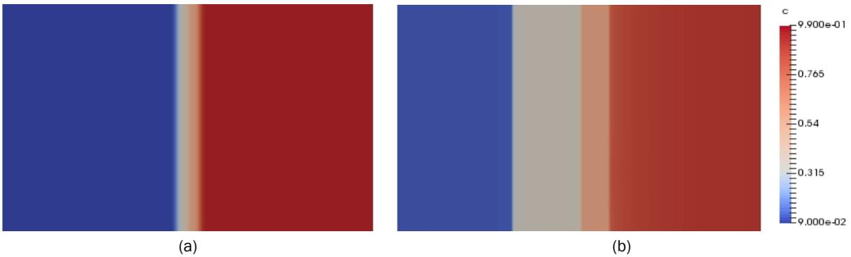
Figure II.3.2.16. PF model of IMC layer growth in diffusion-bonding for (a) the initial condition and (b) after significant growth. The scale bar on the right shows Mg mole fraction. Note the faster growth of  $\text{Al}_3\text{Mg}_2$  (grey) than  $\text{Al}_{43}\text{Mg}_{57}$  (pink) as seen in the experiments. Source: WPI.
