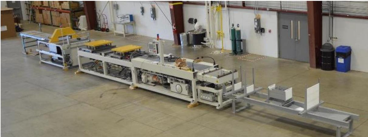
Figure II.2.10.8. Strongwell pultrusion equipment at the CFTF. Source: ORNL.
