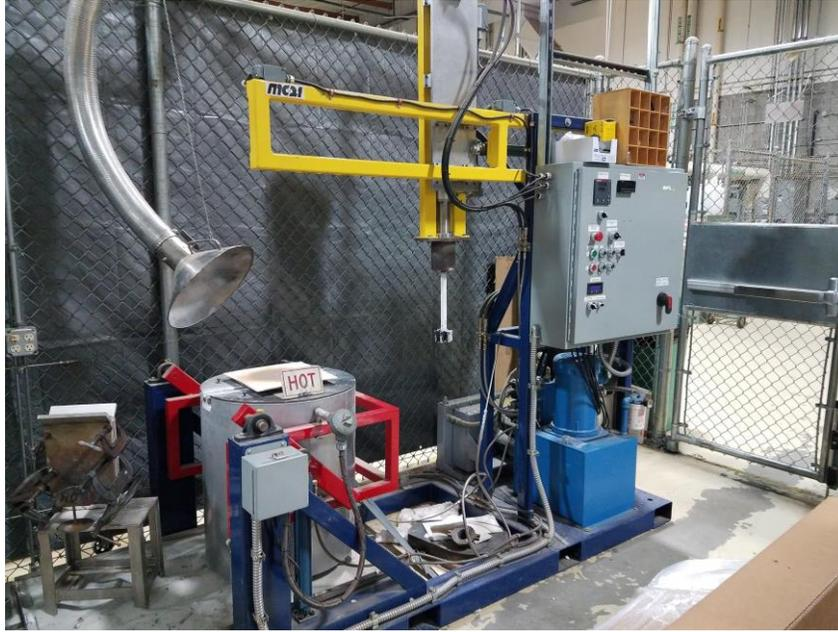
Figure I.2.2.2. PNNL tilt-pour stir-casting equipment used for the casting trials. Flat-bladed impeller installed in mixer head.
