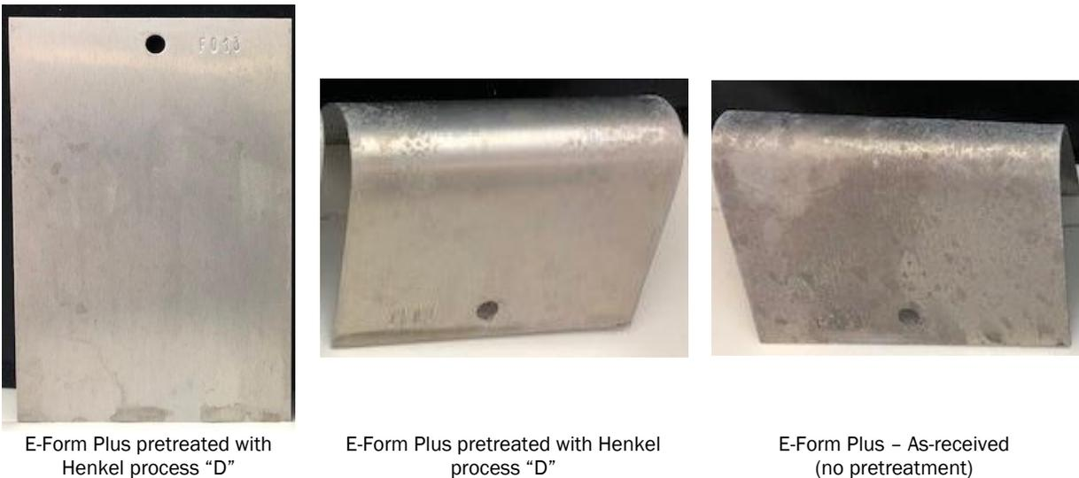
Figure II.1.2.23. Bend test after humidity exposure showing no apparent increase in oxidation. Source: Henkel.
