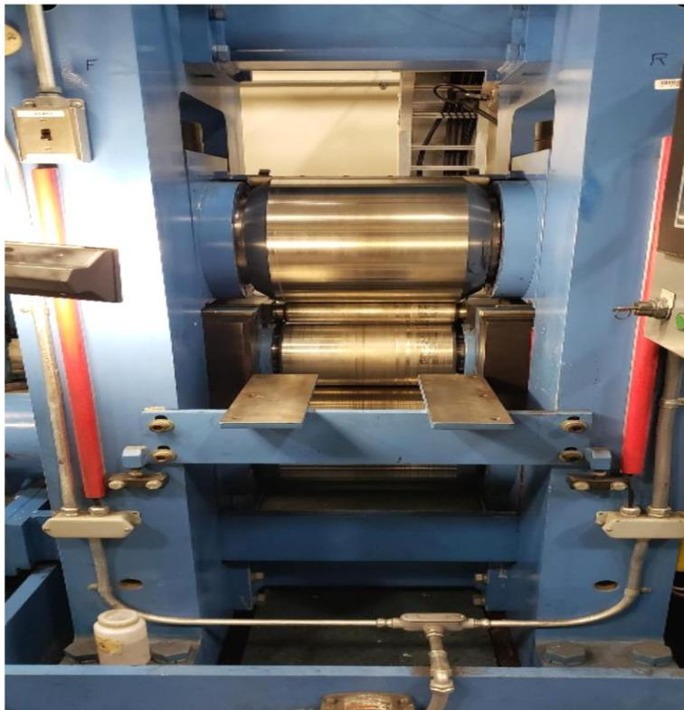
Figure II.1.2.5. Shear roll arrangement for asymmetric rolling. Source: ORNL.
