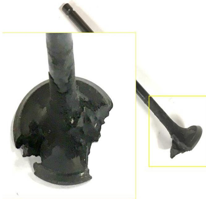
Figure I.1.5.1. Extreme environmental degradation to an alloy 21-4-3 valve head due to local temperature spikes resulting from improper seating. Source: Tenneco.
