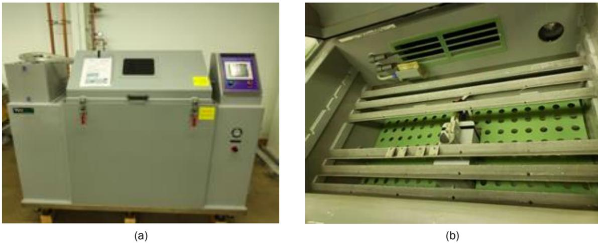
Figure II.3.2.9. (a) WeiCe CCT equipment; and (b) corrosion chamber with samples. Source: WPI.
