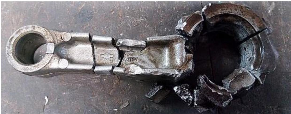
Figure I.3.5.4.1. Al connecting rod for a 4-stroke engine failed by fatigue, which subsequently impacted the crankshaft and caused catastrophic engine damage. Source: Wikipedia.
