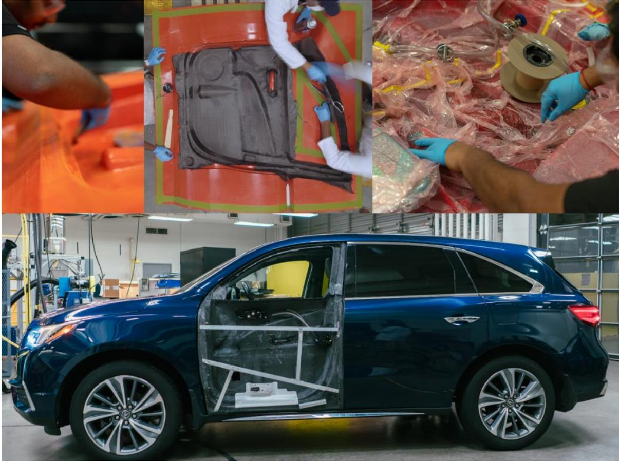
Figure II.2.4.16. Composite door manufacturing process. Source: Clemson University.
