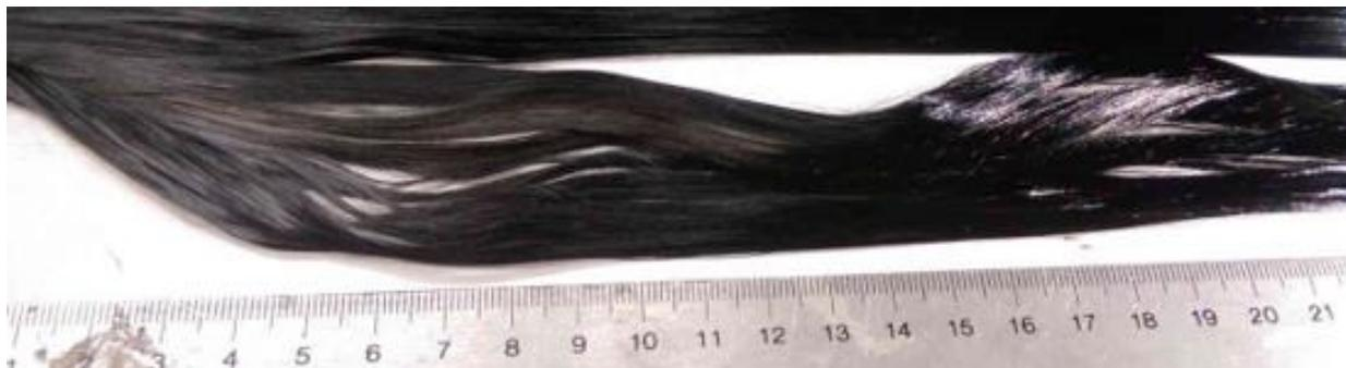
Figure II.2.11.2. A bundle of several hundred of grey filaments between 10 mm and 120 mm was found among the 8 tows of the static batch. Its total length was measured to ca. 8 in. Source: 4XTechnologies.
