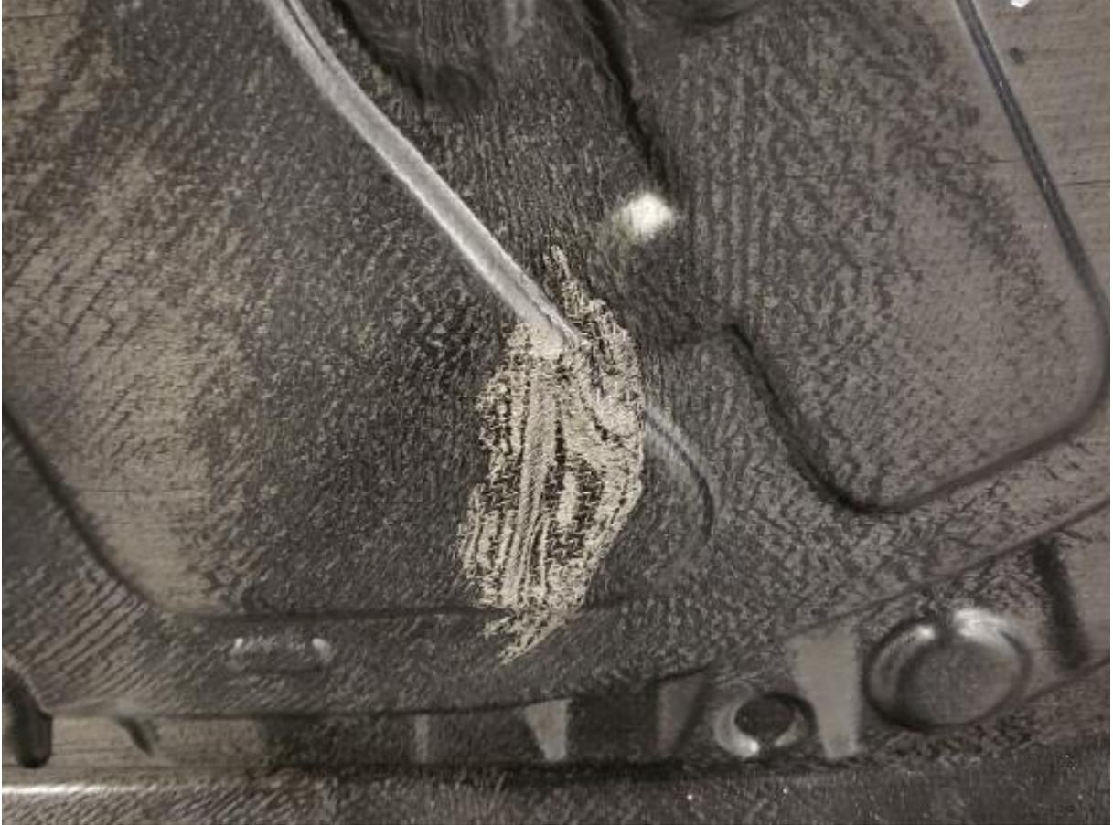
Figure II.2.3.20. Dry area. Source: TPI Composites.
