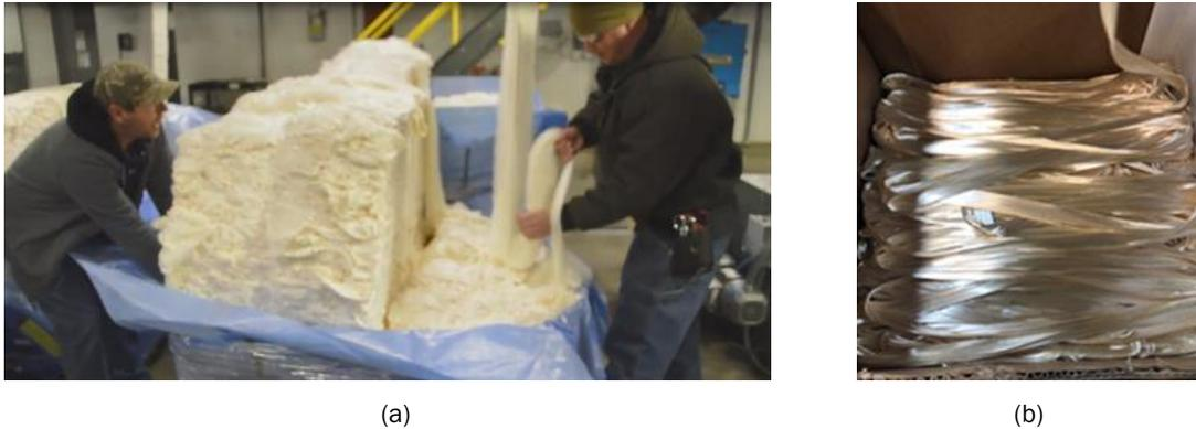
Figure II.2.10.3. (a) Old packaging method that was bulky and time-consuming; and (b) new simplified packing configuration. Source: ORNL.
