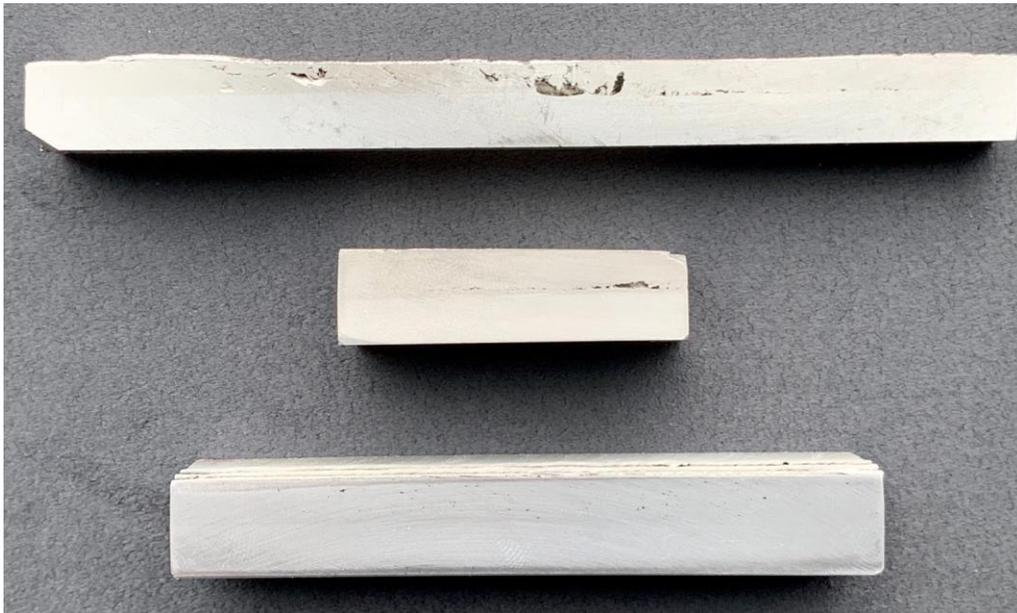
Figure I.3.5.3.3. Progressive process refinement to achieve fully dense consolidated material blocks for property testing. Source: ORNL.
