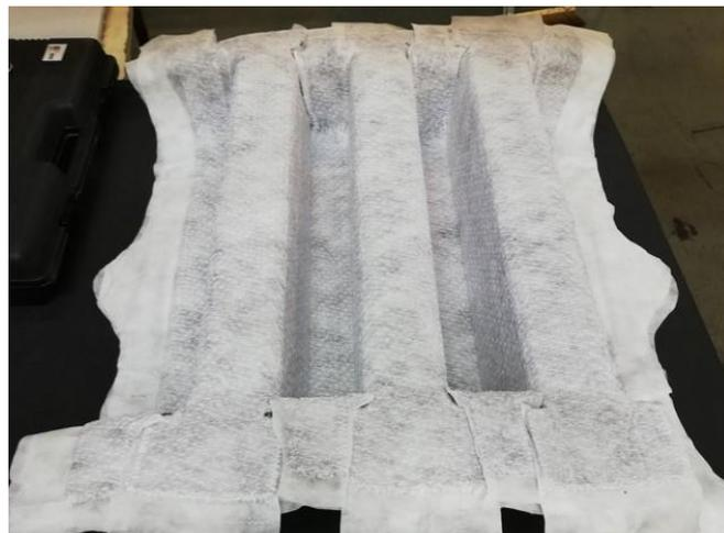
Figure II.2.5.16. Coats 3D preform. Source: GM.
