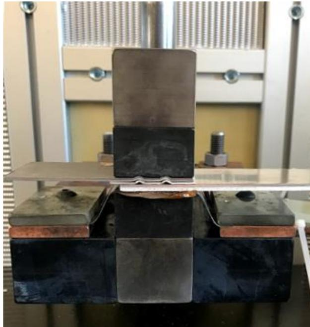
Figure II.3.4.11. (a) A pre-prototype system and (b) a closer view of the pre-prototype welding head #1. Source: OSU.
