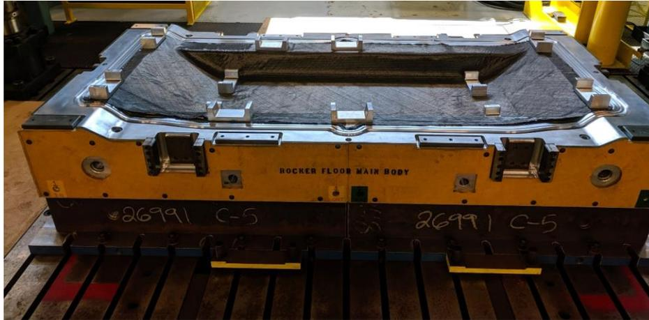
Figure II.2.5.21. Floor preforming pattern for the main blank, draped on the tool. Source: GM.
