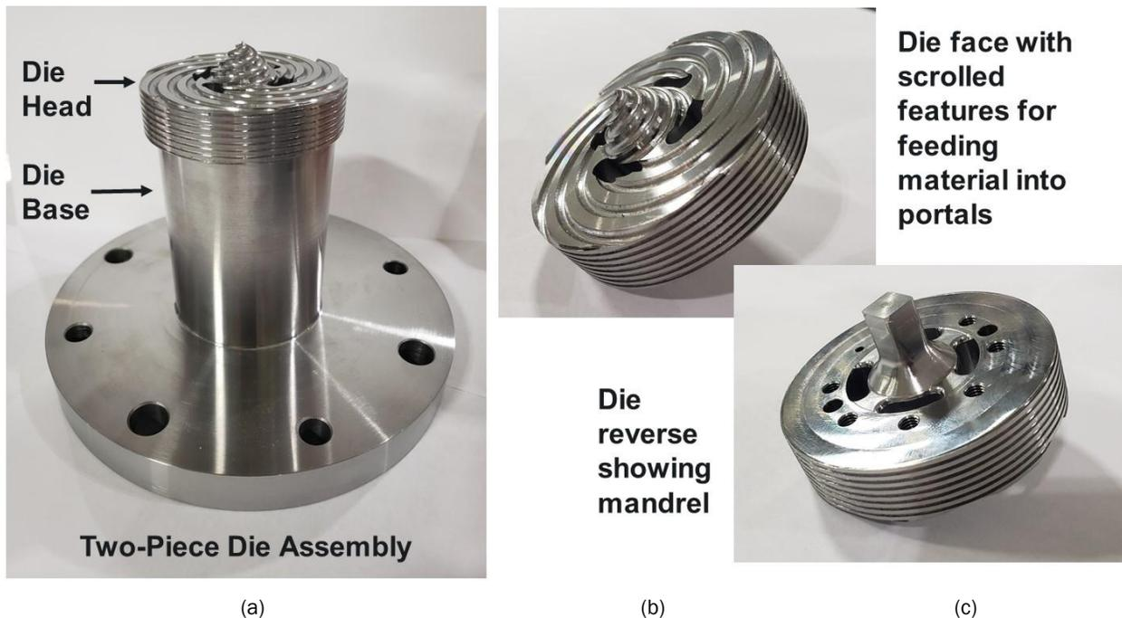
Figure II.1.1.3. (a) Two-piece portal bridge die design showing: (b) scrolled-face (front side); and (c) mandrel (back side). Source: PNNL.
