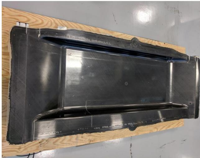
Figure II.2.5.22. Example of an untrimmed floor. Source: GM.
