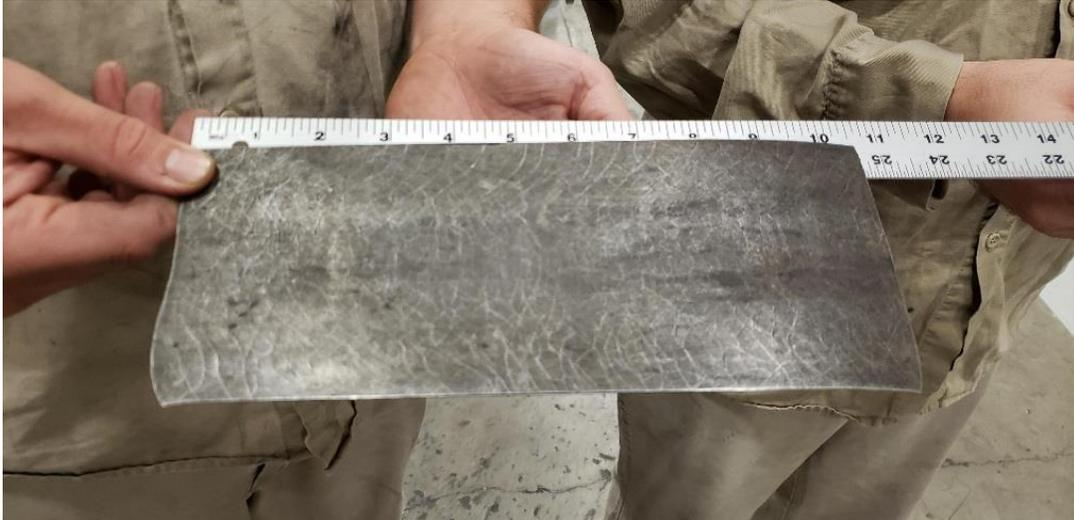
Figure II.1.2.4. ORNL-rolled Alloy 2 Plus sheet (size is ~1.65-mm-thick and ~11-cm wide). Source: ORNL.
