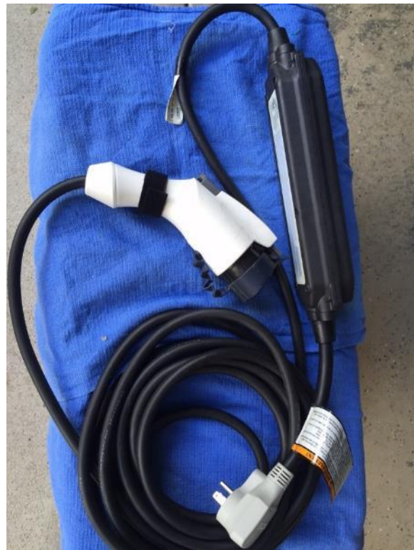
Photo 6. A Level 1 charging cordset comes standard with most PEVs and allows a driver to use Level 1 charging receptacles. Photo from Erik Nelsen, NREL 34792
