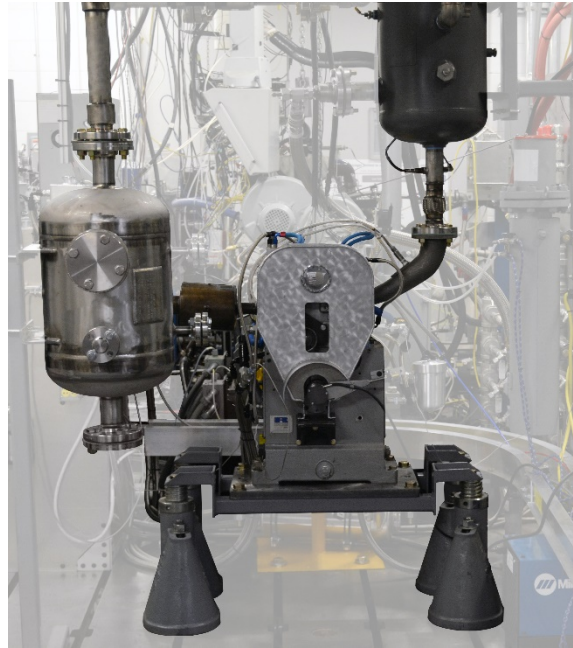
Figure II.3.2 Picture of the new single-cylinder engine installation at ORNL, supported by GM, to investigate multimode combustion for Co-Optima
