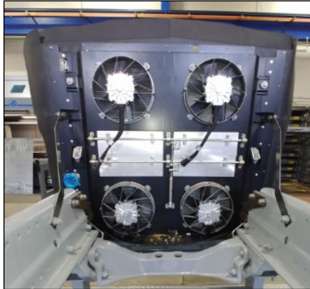
Figure V.2.2 Powertrain mule WHR cooling module with integral electric fans and louvers
