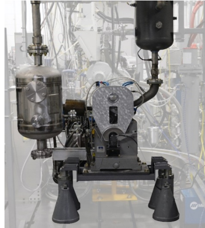
Figure 7 The new single-cylinder engine at ORNL, used to investigate multimode combustion for Co-Optima (Szybist, II.3)
