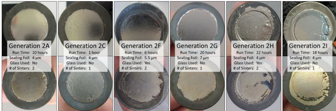
Figure V.8.3 Pre-test (top) and post-test (bottom) condition of coated valves
