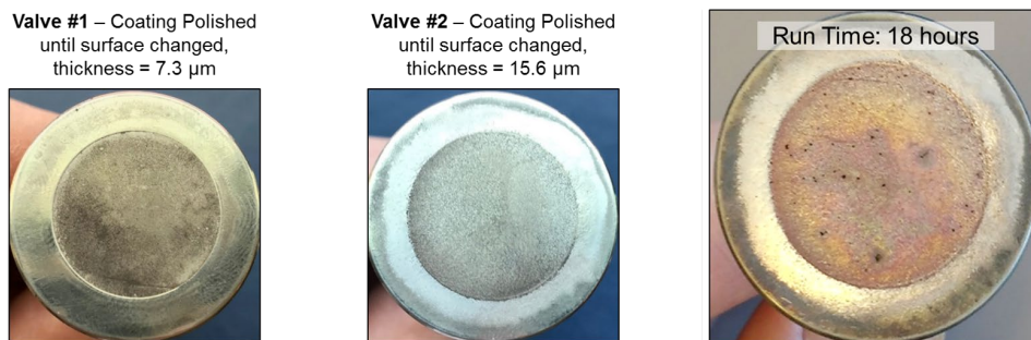
Figure V.8.4 Ceramic sealing layer exhaust valve images and thicknesses; far right: valve #2 after 18 h engine testing
