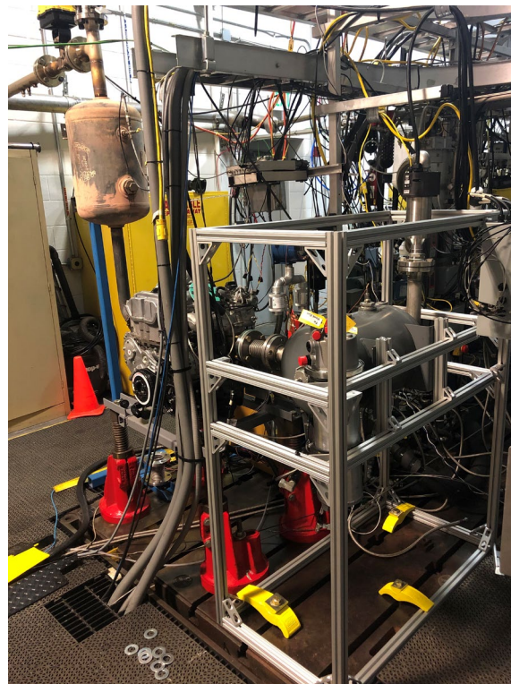
Figure II.8.4 Dry sump single-cylinder LNF engine installation and conversion
