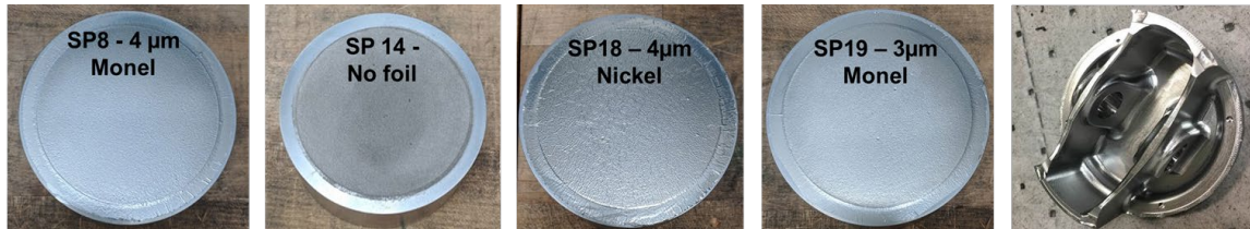
Figure V.8.5 Insulating and sealing layer configurations on steel pistons: top view and underside machined view
