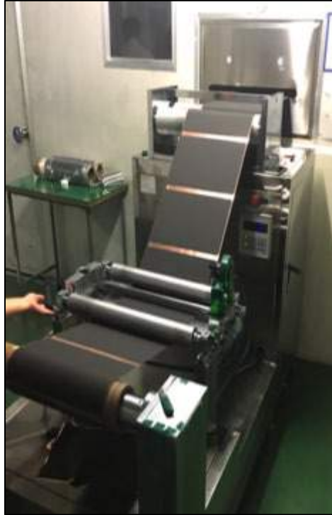
Figure I.1.C.4 NanoGraf anode coating on pilot-scale equipment with 4mAh/cm 2 and 10wt% binder content
