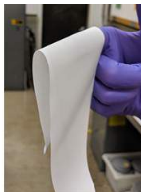
Figure I.2.M.3 (Left) Tape casting dispersant optimization and (right) photograph of optimized LLZO tape
