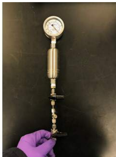
Figure II.3.G.8 Custom gas manifold control plate (left) is comprised of a series of needle and ball valves, and monitored using the digital pressure gauge ( \pm .1 torr). A typical sample cylinder containing the desired mixture allows for the direct sampling of the gas without contaminating the bulk mixture (right)
