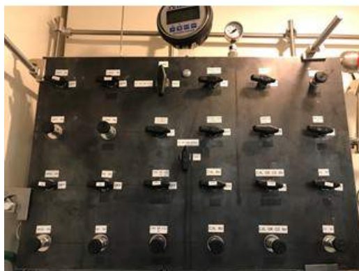
Figure II.3.G.8 Custom gas manifold control plate (left) is comprised of a series of needle and ball valves, and monitored using the digital pressure gauge ( \pm .1 torr). A typical sample cylinder containing the desired mixture allows for the direct sampling of the gas without contaminating the bulk mixture (right)
