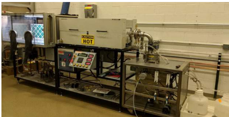
Figure II.4.A.1 Reactive spray technology system set up and optimized at ANL to produce cathode material
