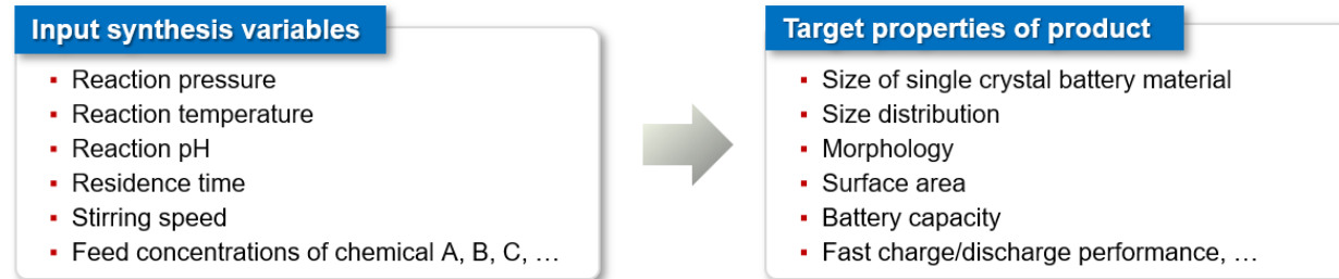
Figure I.2.G.2 Optimization of synthesis variables to achieve final target properties of battery materials
