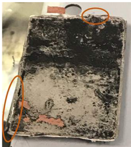
Figure II.12.A.23 Post-test Li metal electrode at the completion of 200+ cycles. Circles indicate areas of disconnected Li after cycling
