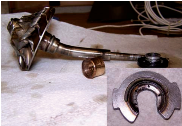
FIGURE 2. Catastrophic Failure of the First Prototype Turbocharger due to Overloaded Thrust Bearing
