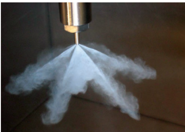
FIGURE 2B. Second Phase Injection with Multi-Jet Spray and Wide Spray Angle
