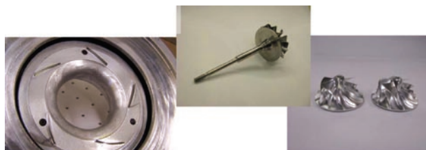
FIGURE 1. A Mixed Flow Turbine Wheel was Fabricated as Well as Ultra-Low Solidity Airfoil Diffuser Vane Compressor
