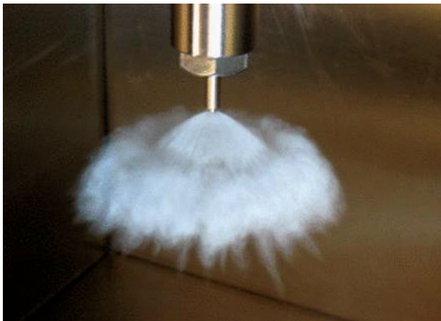
FIGURE 2A. First Phase Injection with Conical Spray and Narrow Spray Angle
