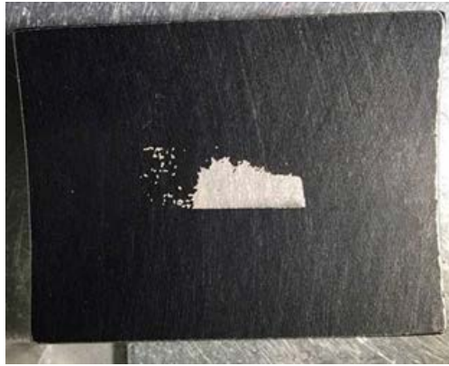
Figure II-30: A cast-iron liner segment coated with a DLC coating from C2D showing delamination.
