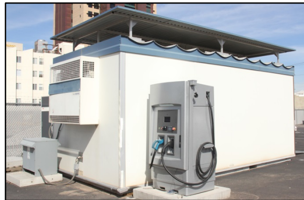
Figure II-18: Vehicle temperature chamber with Advanced Charging Technologies DCFC configured with both CHAdeMO and combined charging system connectors located at Intertek in Phoenix, Arizona.
