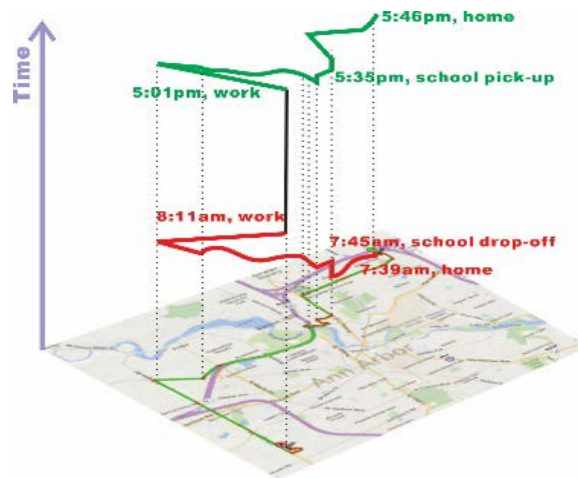
Figure II-21: Example time-space trajectory extracted from the Safety Pilot Model Deployment Database
