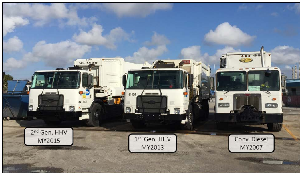
Figure III-27: Three configurations of refuse trucks from which data were collected
