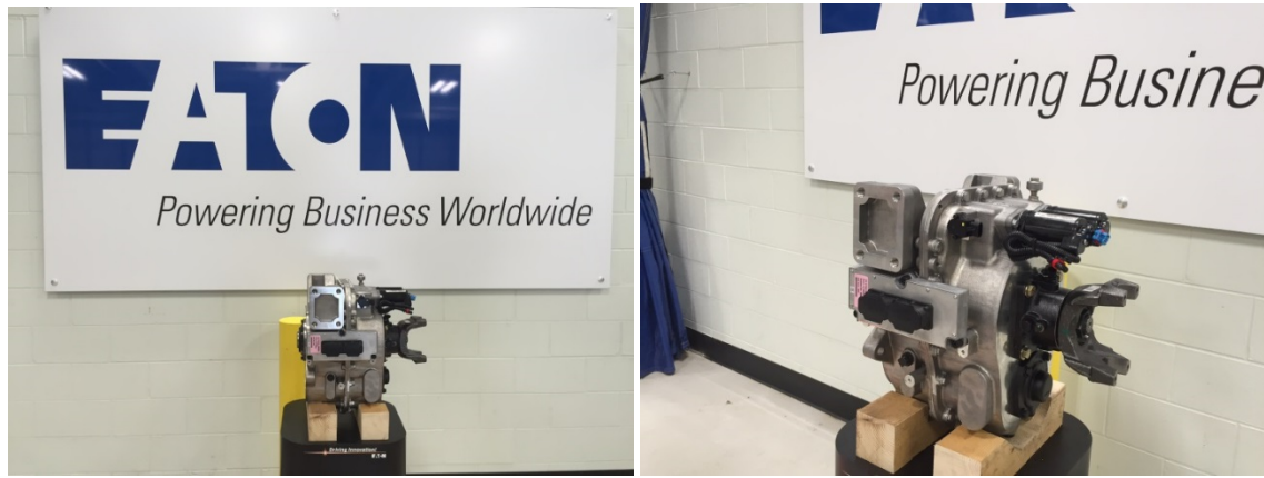
Figure II-14: The display unit of the new 4-speed EV Transmission.
