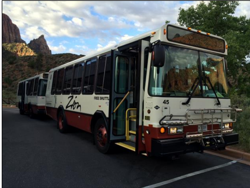
Figure III-63: Zion NPS propane-powered bus connected to a non-powered passenger trailer
