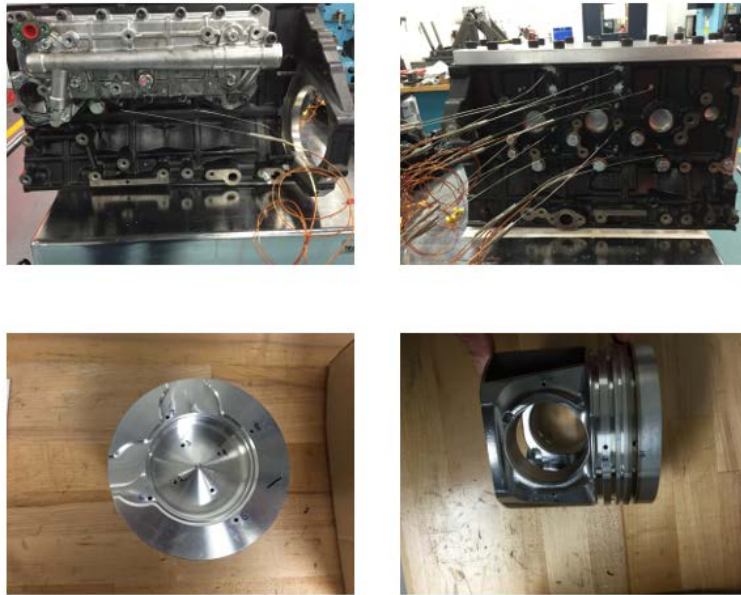
Figure II-51: Instrumented block with thermocouples (top) and piston with templugs (bottom).
