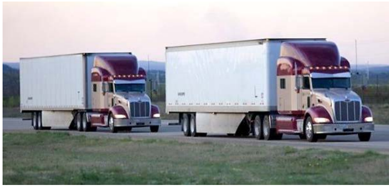
Figure VI-17: Trucks in platoon formation during testing
