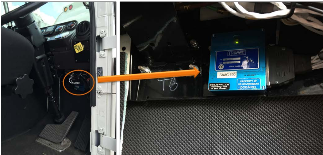
Figure III-28: Installation location of on-board Isaac data logger Photo by Robert Prohaska/NREL
