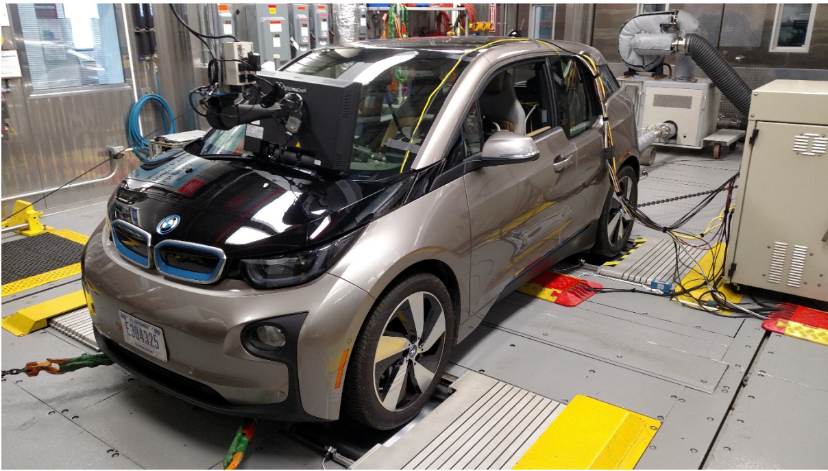
Figure III-91: 2014 BMW i3 REx mounted in APRF for evaluation.
