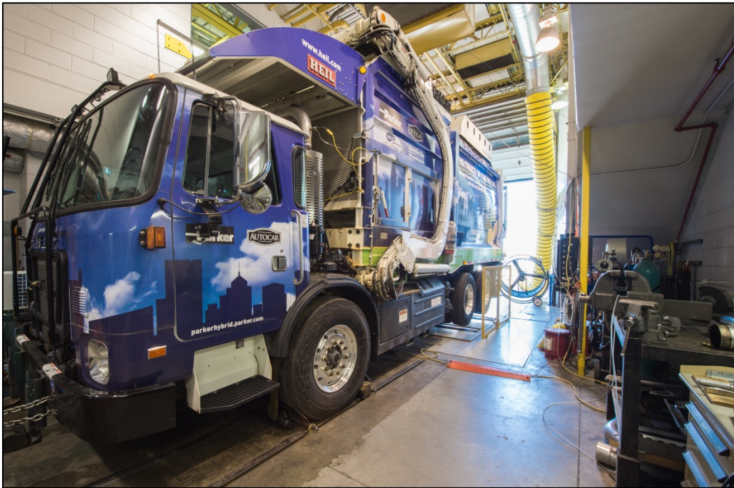
Figure III-39: 2013 AutoCar E3 MY15 HHV refuse truck with Cummins ISL-G engine at NREL's ReFUEL laboratory Photo by Dennis Schroeder / NREL 38576
