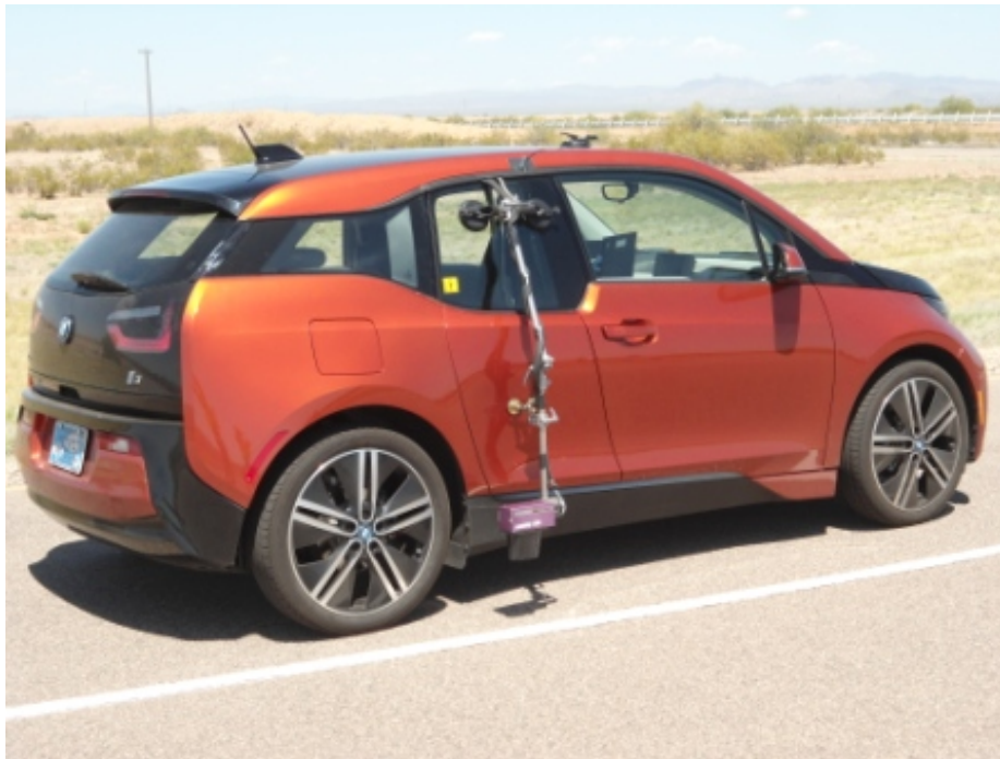
Figure III-2: A 2014 BMW i3 electric vehicle fitted with testing and measurement equipment for track testing.
