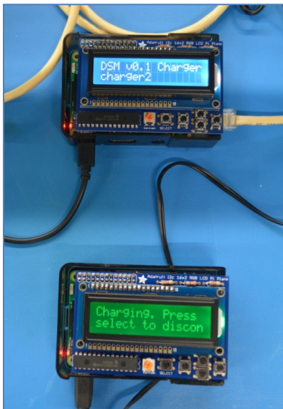
Figure VI-83: The DSM Prototype Hardware and Software - Showing 2 EVSE DSM Nodes (Blue) and a PEV Node (Green) Connected to EVSE #2. The BEMS Displaying the Status of the DSM Framework
