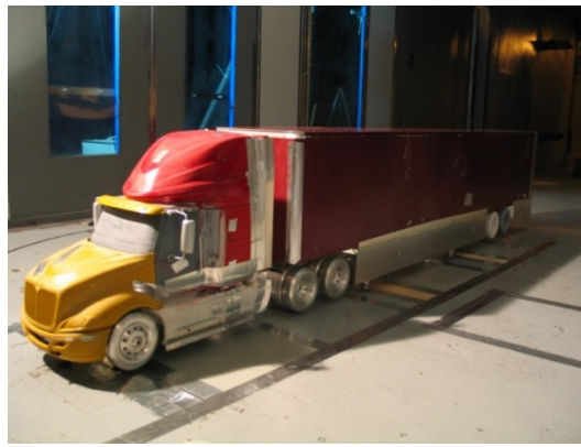
Figure VI-1: Baseline heavy vehicle model (1/8th scale) in the NASA Ames 7x10 wind tunnel
