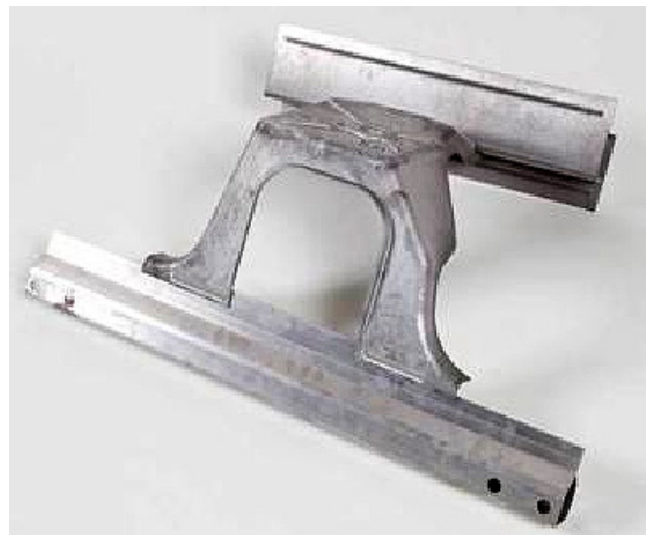
Figure 1. Friction-stir-welded all-magnesium demonstration subassembly comprised of a central AM60B die casting, AZ31 sheet-formed upper box, and extruded AM30 lower rail.
