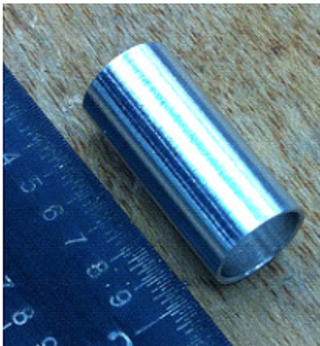
Figure 1. Mg alloy tubular sample used to evaluate energy absorption capacity in a compression test.
