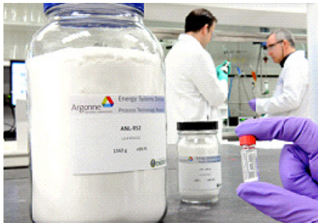
Figure 1. Container of the DBBB overcharge shuttle additive scaled-up from 1 gram to kilogram quantities for commercial testing.
