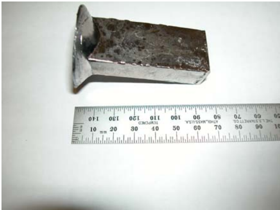
Figure 4. Small heats of alloys were melted and cast in a vacuum arc furnace, homogenized, aged, and specimens were machined for high temperature tensile tests.
