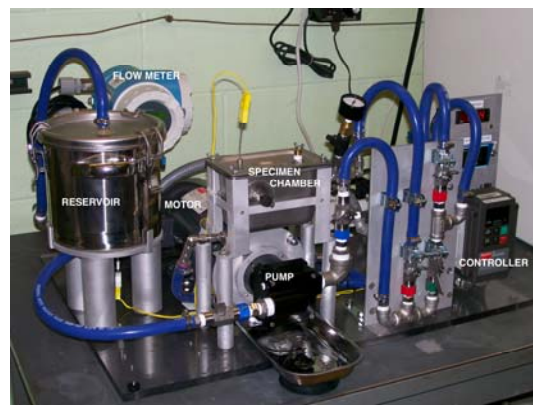
Figure 1. Photograph of the liquid erosion apparatus.
