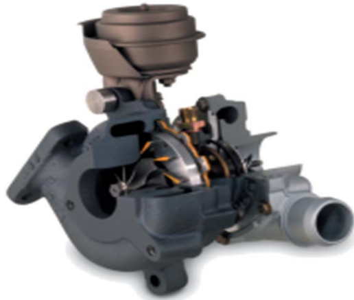
Figure 2 – Typical Honeywell turbocharger system for passenger vehicles. Cut-away shows turbine wheel inside the cast-iron casing (nearest end) of the turbine end, an aluminum housing on the compressor side, and the transition region in between, containing the steel shaft connecting both wheels and bearings.
