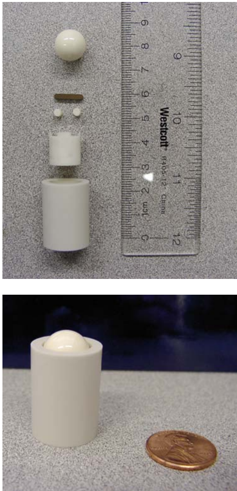
Figure 7. High temperature three-point bend fixture designed for testing small prismatic bars of thermoelectric specimens.
