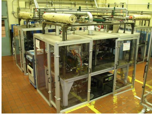
Figure 6. Thermo-mechanical valve and seat-insert test rigs for simulating high-temperature wear and performance of exhaust valves and seats for diesel engines, at the Caterpillar Technical Center. Caterpillar completed expanding facility from one to three test rigs this year, and began wear-testing of new modified seat-inserts.
