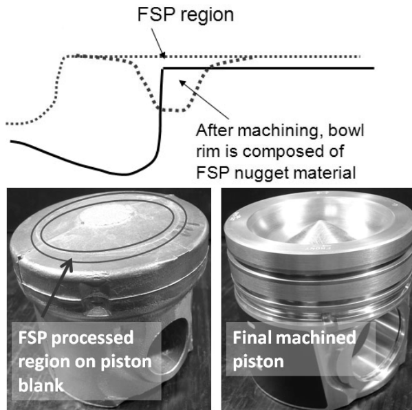
Figure 6. Cast Piston Blank (The area in the bowl rim after machining will be friction stir processed for improved microstructure.)
