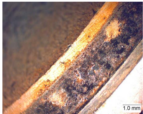
Figure 1. Used diesel engine exhaust valve sealing surface showing the combined effects of corrosion, deformation, and wear.
