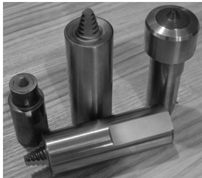
Figure 3. Friction Stir Process Illustration (top) and Typical Friction Stir Tools
