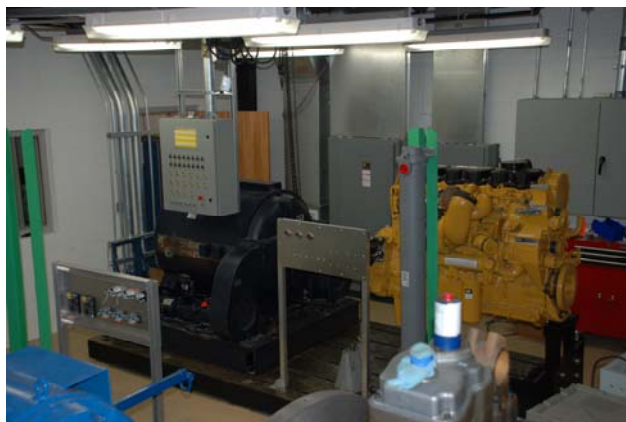
Figure 10. Photograph showing mounted engine and dynamometer. The control room is on the other side of the wall on the left of the photograph and behind the dynamometer.
