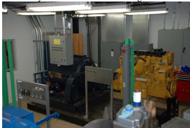
Figure 1. Photograph showing mounted engine and dynamometer. The control room is on the other side of the wall on the left of the photograph and behind the dynamometer.
