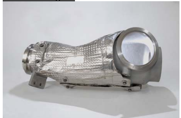
Figure 1. Caterpillar Regeneration System (CRS) burner housing, made of CF8C-Plus cast stainless steel, for regenerating ceramic diesel particulate filter (DPF) components. Commercial application began in late 2006, and to date over 450 tons of CF8C-Plus steel have been cast. CRS units, attached to the turbocharger, must endure rapid thermal cycling for maximum temperatures close to 900°C. No CRS units have failed, with the longest service being 3 years or more.
