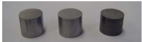
Figure 9. N-type and p-type Skutterudite ingots produced by the SPS method.
