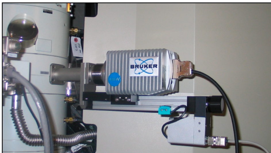
Figure 4. A new silicon drift x-ray detector, desired for inherently give low count rate environments, was installed on the ACEM.
