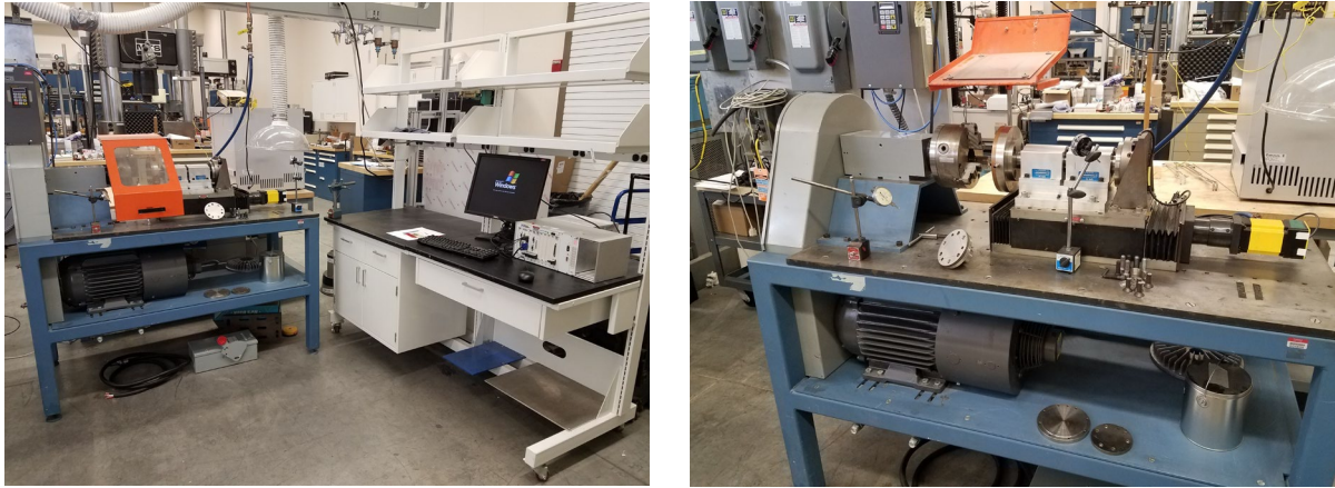
Figure I.3.B.5. Brake-friction pair test-stand at PNNL. Source: PNNL.
