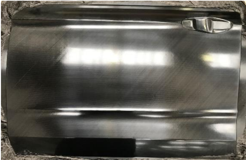
Figure II.4.C.12. Finished molded outer door. Source: TPI Composites.
