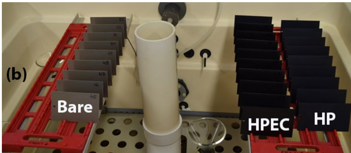
Figure II.3.J.1. (a) Salt-fog test setup at PNNL; (b) Bare and coated (HP and HPEC) AZ31 coupons ready for testing. Source: PNNL.
