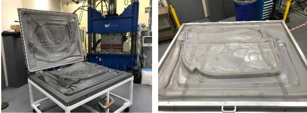
Figure II.4.C.6. Inner door preform tool with (a) placing pre-consolidated ply stacks in a mold; and (b) cured finished part. Source: TPI Composites.
