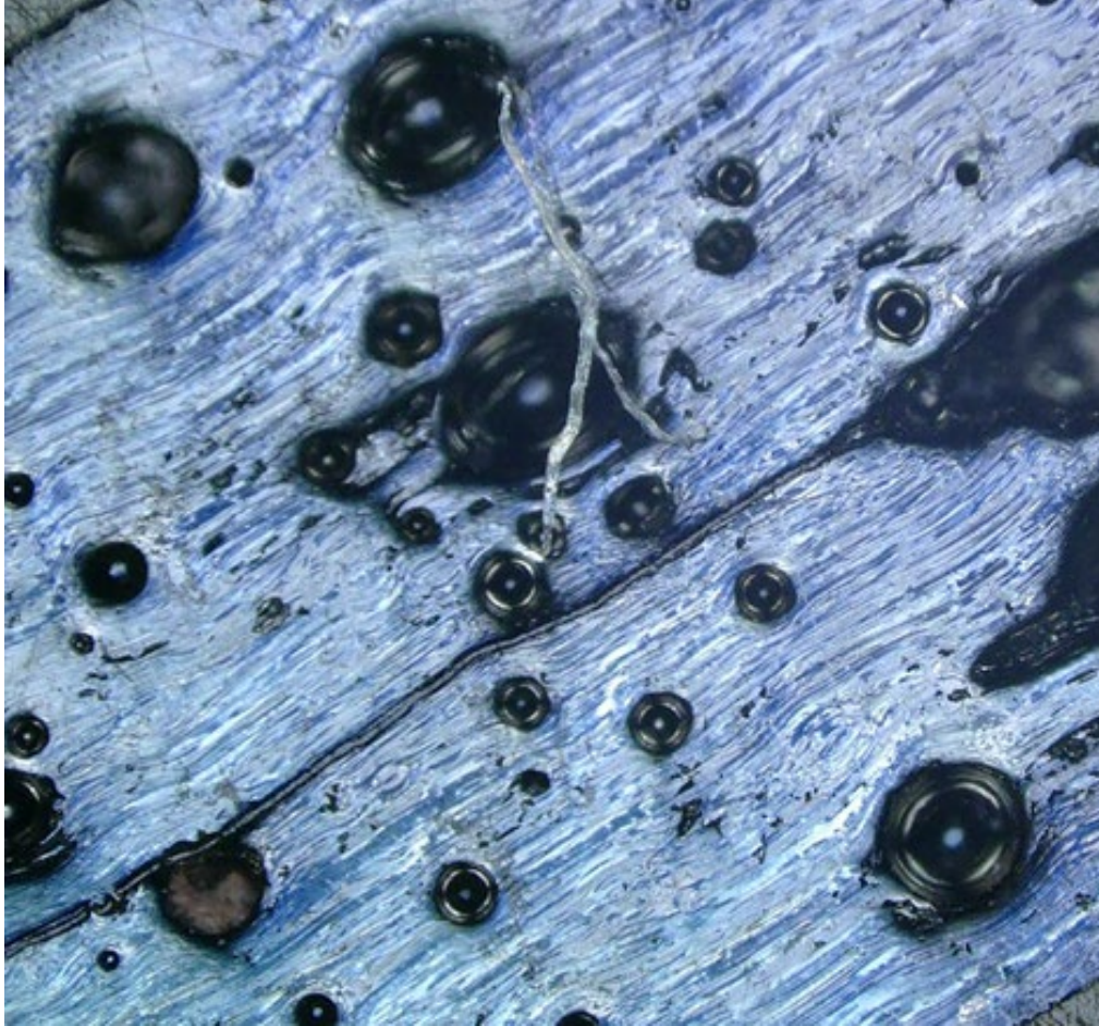
Figure II.2.F.5. Cross-polarized light optical microscopy micrograph showing 95+% mPP produced from M50 iPP by ACP. Source: WRI.
