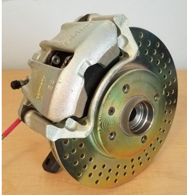
Figure I.3.B.1. Conventional brake design utilizing an Al caliper and a cast-iron brake disc. Source: PNNL.
