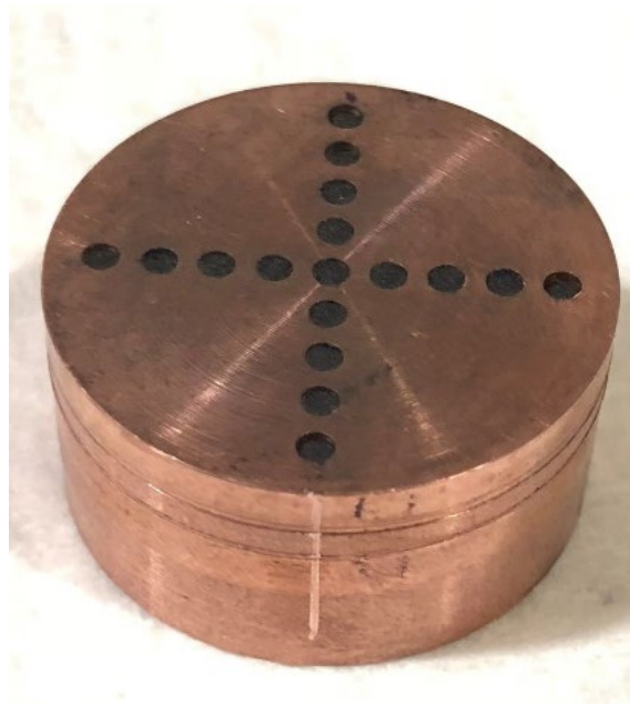
Figure I.3.C.4. Cu cylinder drilled and filled with C powder Source: PNNL.
