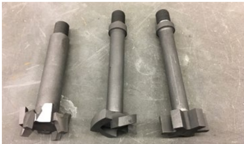
Figure I.3.B.4. Impeller designs for mixing trials. Source: PNNL.
