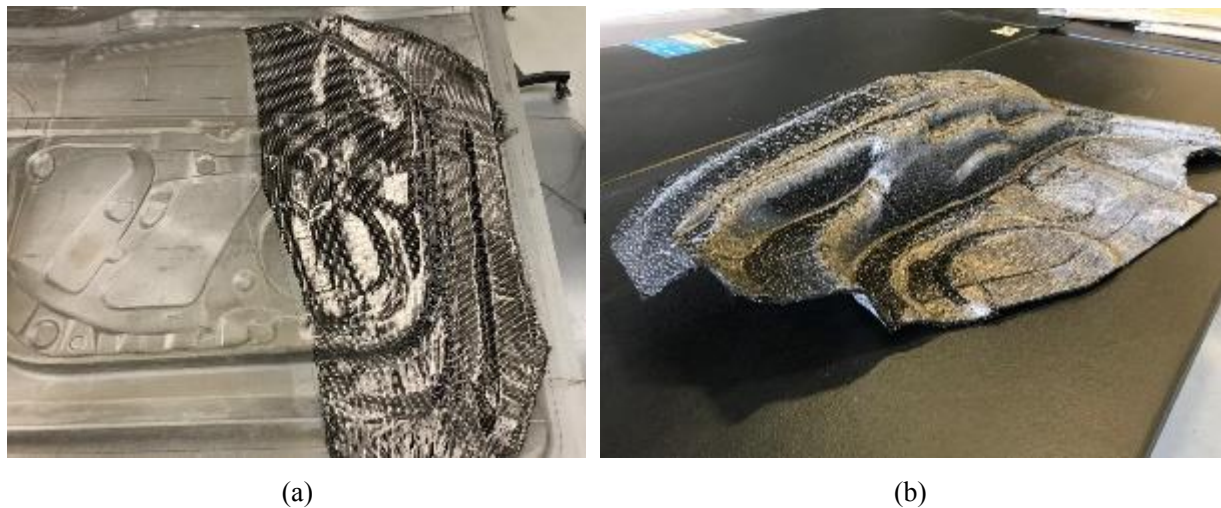
Figure II.4.C.14. Preform fabrication showing (a) preform on the mold; and (b) preform after consolidation and trimming. Source: TPI Composites.
