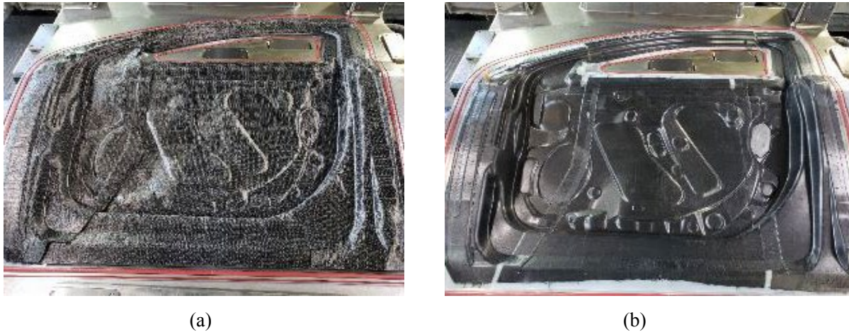
Figure II.4.C.19. Inner door in tool with (a) dry preforms; and (b) molded part. Source: TPI Composites.
