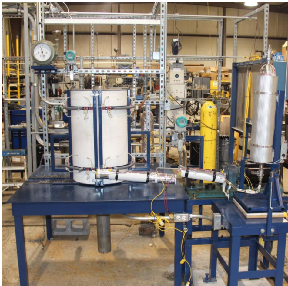
Figure II.2.F.4. A photograph of the ACP 10 continuous pitch processing equipment. Source: ACP.
