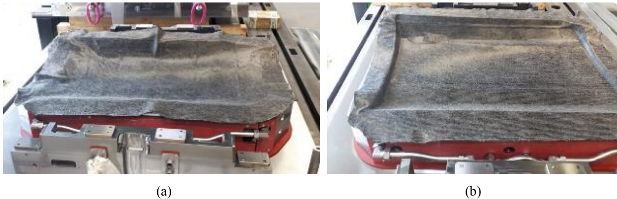
Figure II.4.C.5. Ply pressing trial showing (a) ply stack pre-pressing; and (b) ply stack post-pressing. Source: Alpex.
