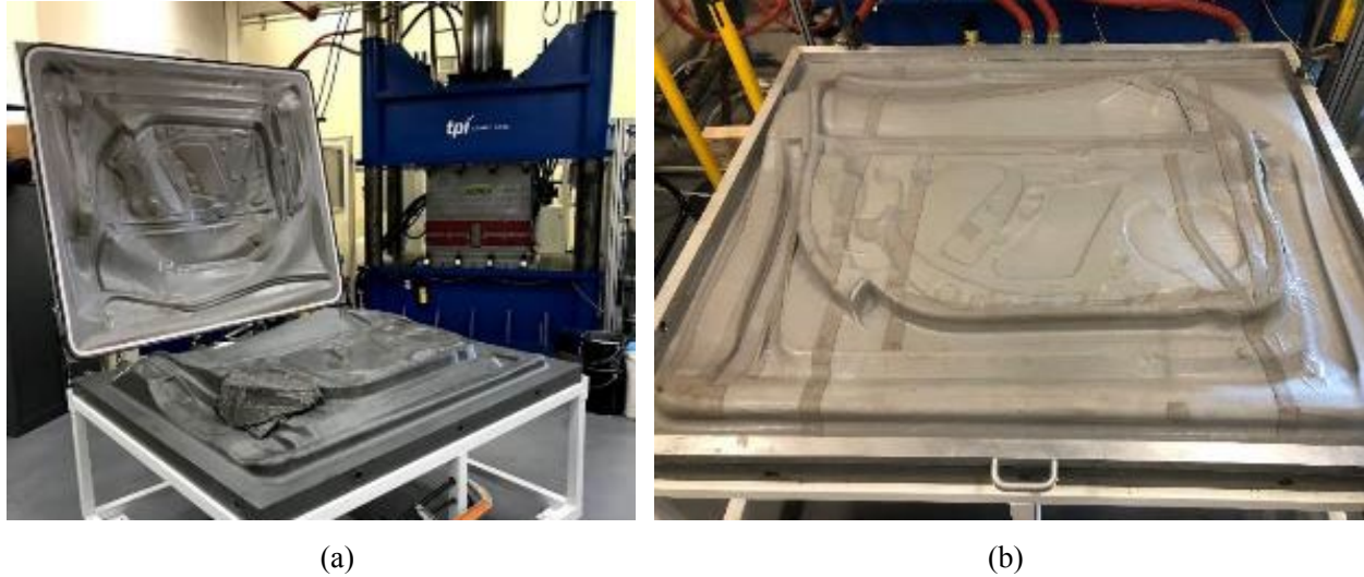
Figure II.4.C.13. Images of (a) the Al preform tool with (b) the silicone vacuum bag. Source: TPI Composites.
