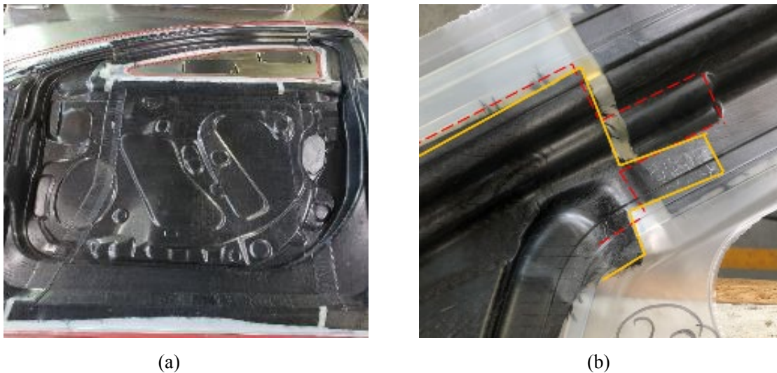
Figure II.4.C.20. Sliding preform at the mirror mount for (a) the area of interest; and (b) at the displaced location. Source: TPI Composites.
