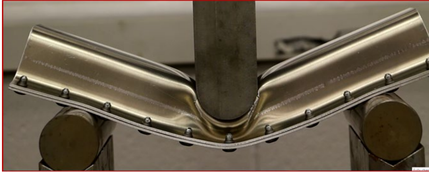
Figure II.1.B.6. Typical performance of samples in a three-point bend test. Source: Cosma.
