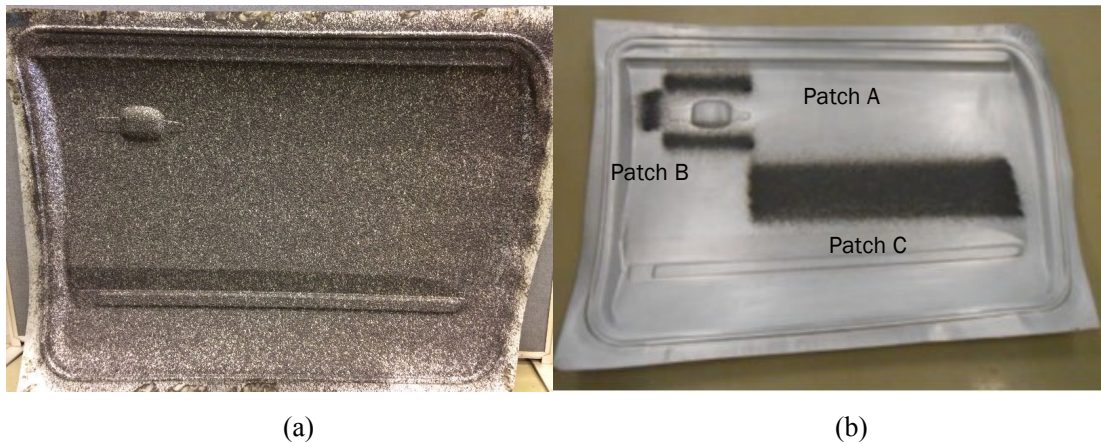
Figure II.1.F.3. Application of the CFRE for (a) total coverage and (b) isolated coverage. Source: ORNL.
