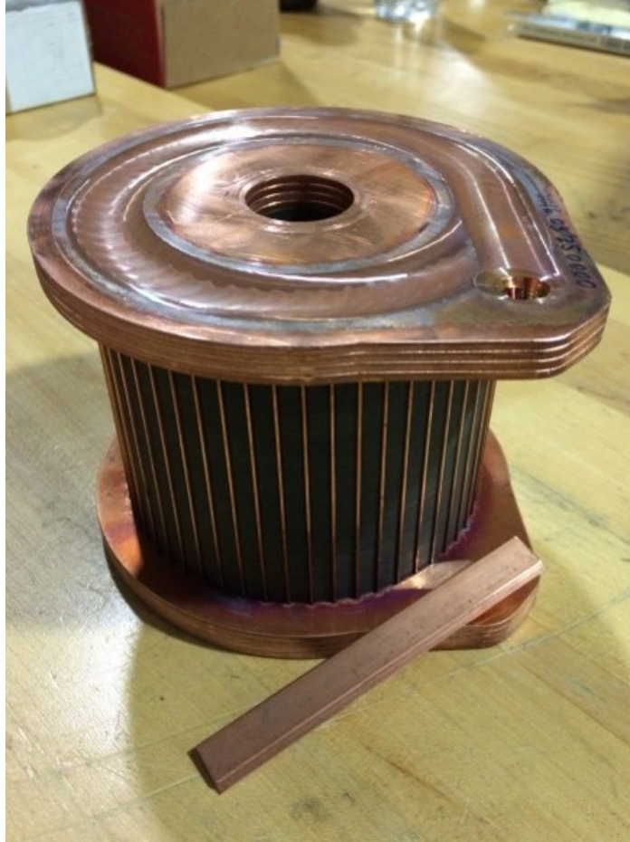
Figure I.3.C.1. Induction motor rotor and an example of a shorting bar. Source: PNNL.
