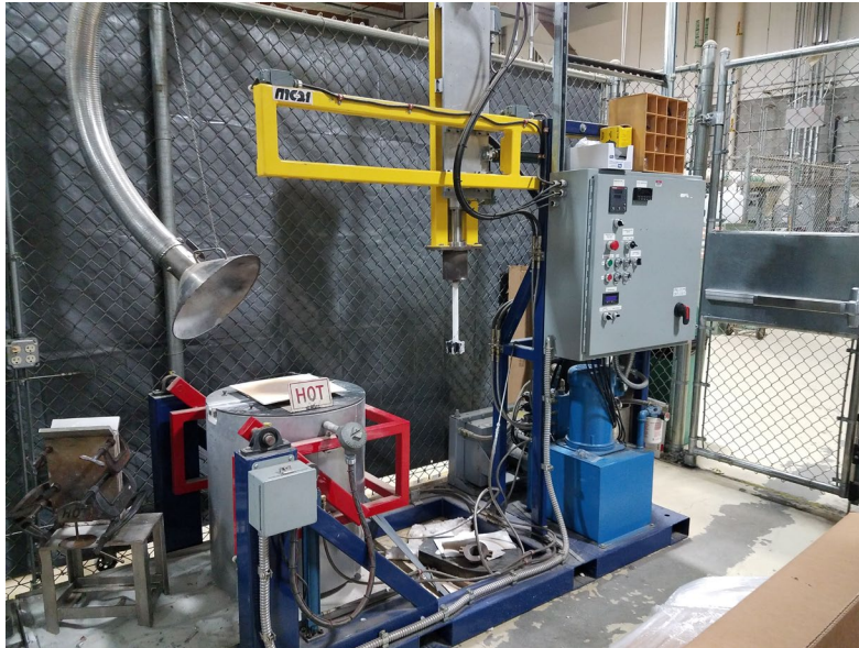
Figure I.3.B.3. Tilt-pour stir-casting equipment at PNNL used for the casting trials. Flat-bladed impeller installed in mixer head. Source: PNNL.
