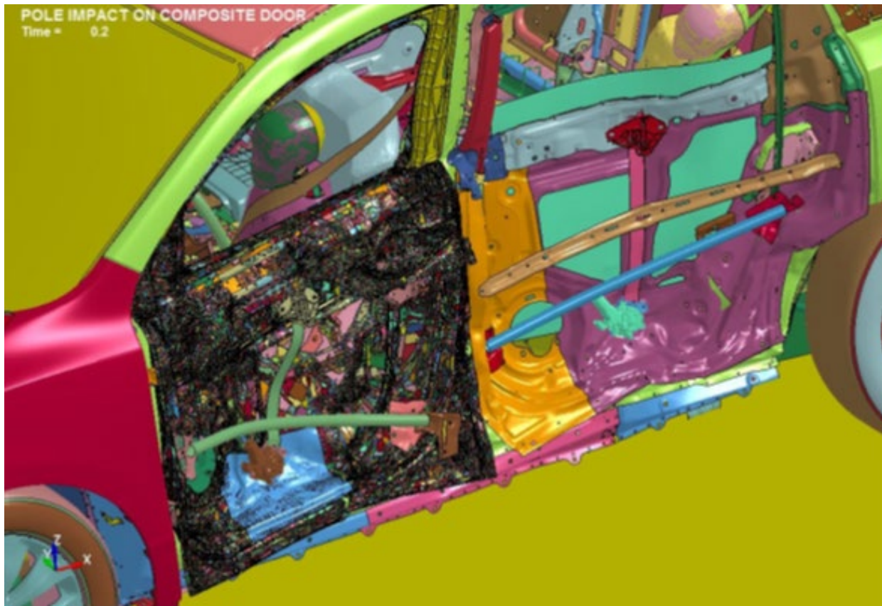
Figure II.4.D.10. Deformation and damage under DB impact conditions. Source: Clemson University.
