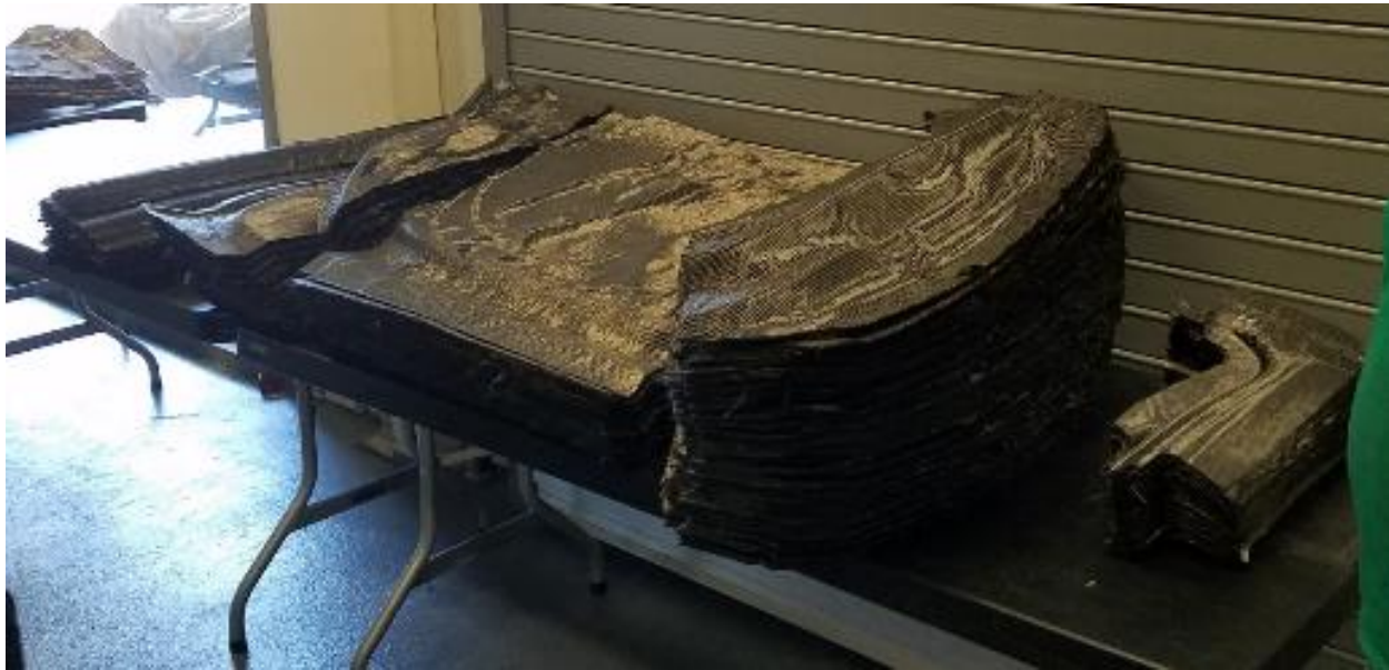
Figure II.4.C.16. Finished preforms ready to ship to Germany. Source: TPI Composites.
