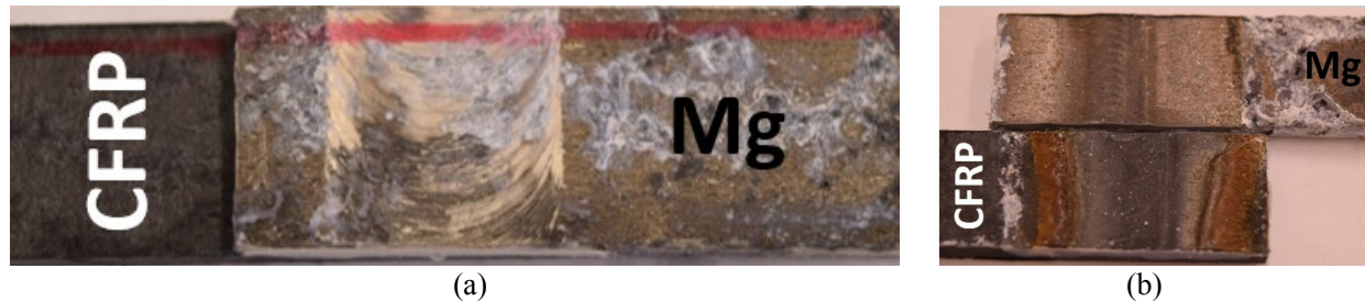
Figure II.3.I.5. Corrosion test with thermal bonding film incorporated. Source: PNNL.
