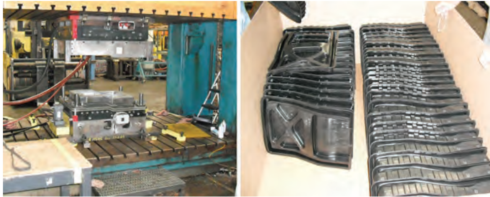
Figure 7. Molding press and tool and molded parts.
