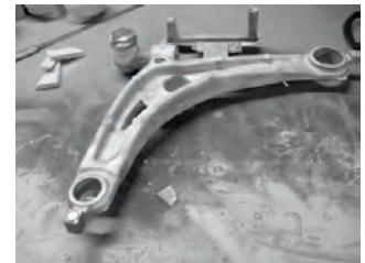
Figure 1. Ablation process: (a) ablation of a mold in progress; (b) ablation of control arm complete.
