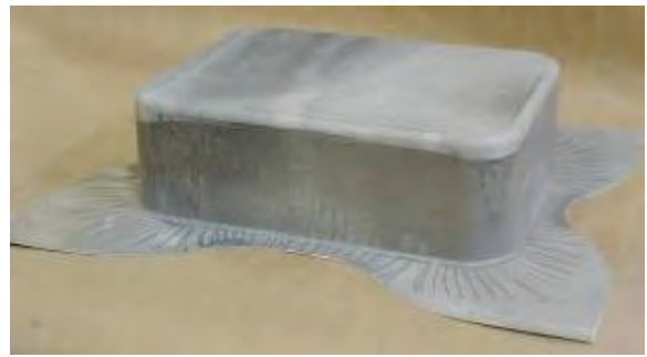
Figure 1. Photograph of the panel formed in the warm forming die in the AMD 602 project.
