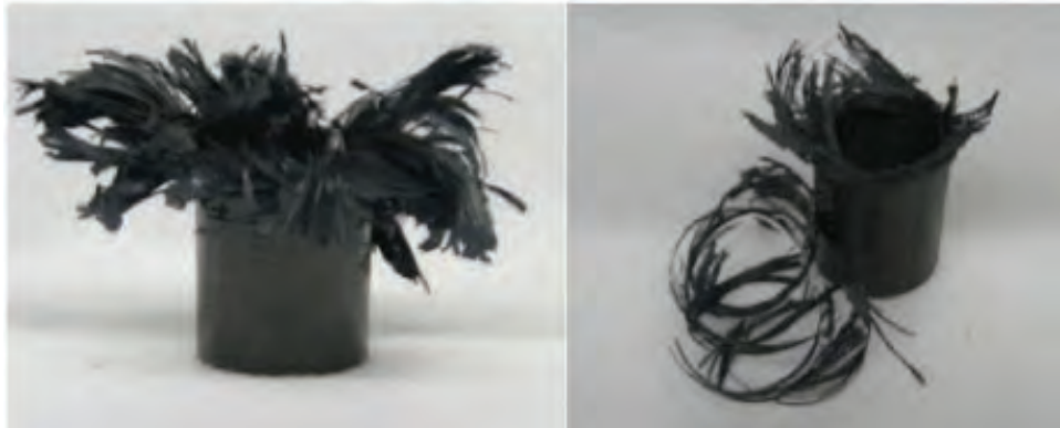
Figure 2. Failure modes produced in circular tube specimens during crush: (a) fiber splaying and (b) fragmentation.
