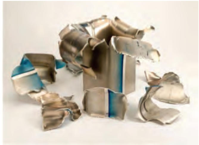
Figure 1. Mg extrusion exhibiting low ductility failure.
