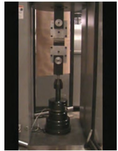
Figure 2. TMAC tension setup for testing the ACC super lap shear weld-bond specimen.
