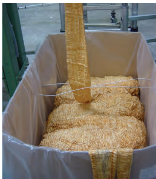
Figure 2. Textile tow precursor as produced by FISIFE and evaluated internally.
