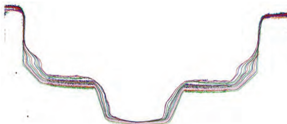
Figure 1. Representative profiles of 70% PCBN tool tip for FSSW of DP980. Wear profiles from 0 to 1200 welds.
