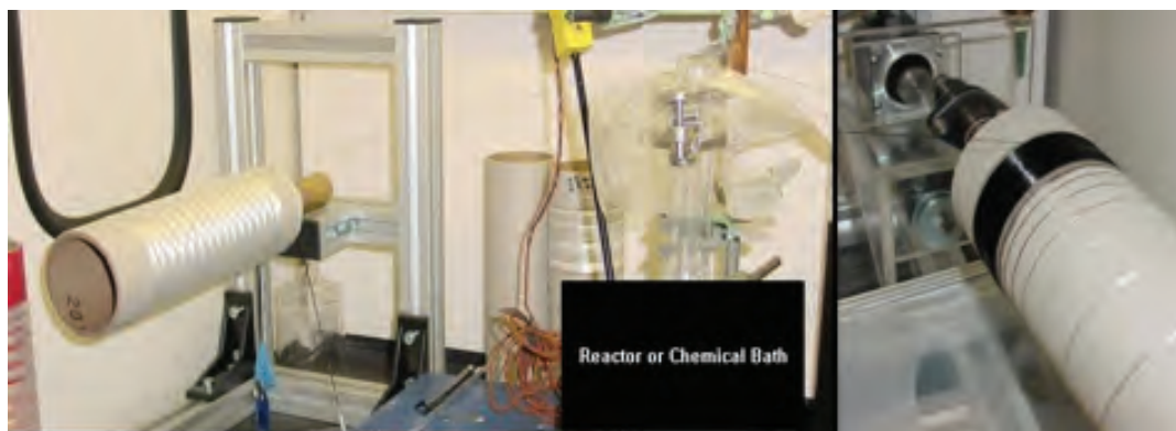
Figure 1. Photograph showing semi-continuous precursor functionalization run.
