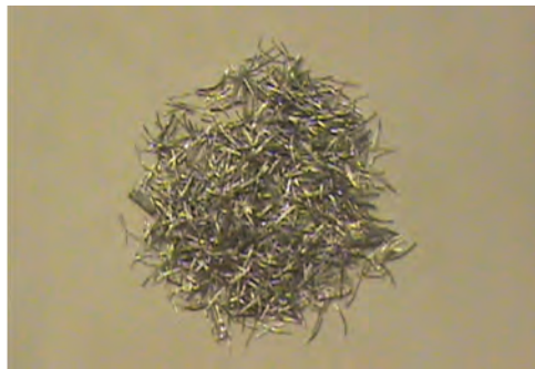
Figure 2. Sample MgAZ31B processed by LSEM. (a) LP LSEM ( p/2k = 1.2 , T = 70^\circ\text{C} ) and (b) HP LSEM ( p/2k = 1.7 , T = 230^\circ\text{C} ). In both cases, \gamma \sim 2 . The deformation zone temperature, T , was achieved naturally, without any work material or tool preheating.
