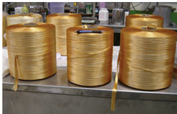
Figure 1. Textile tow precursor as produced by FISIFE and supplied to ORNL on spools for evaluation.
