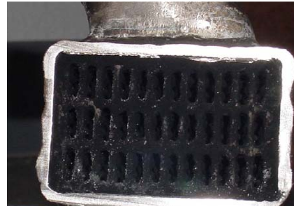
After 200 hr. Fouling Test
