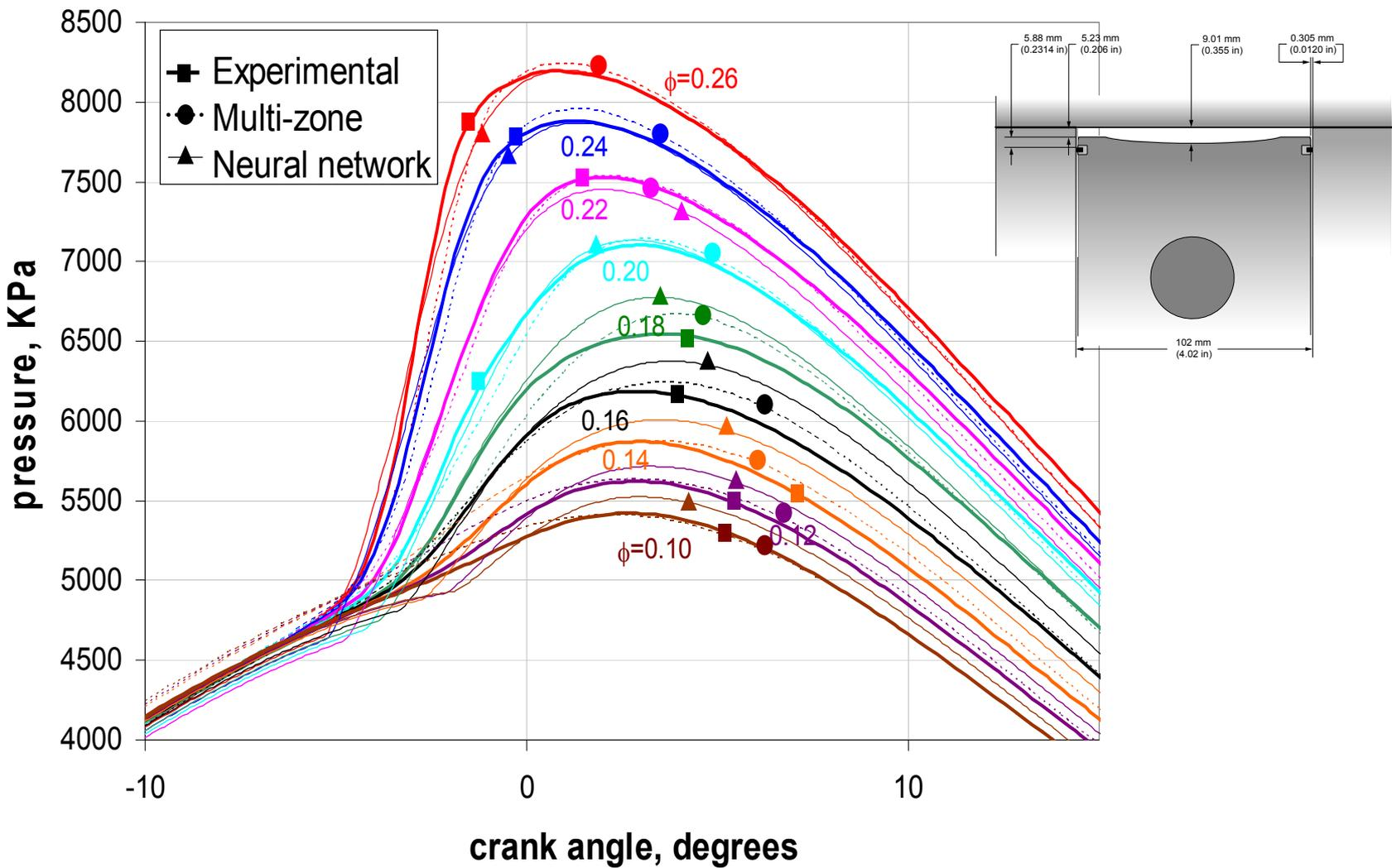
**KIVA-ANN is almost as accurate as detailed kinetic models while considerably reducing computational cost (4 hours for 50,000 element mesh)**
