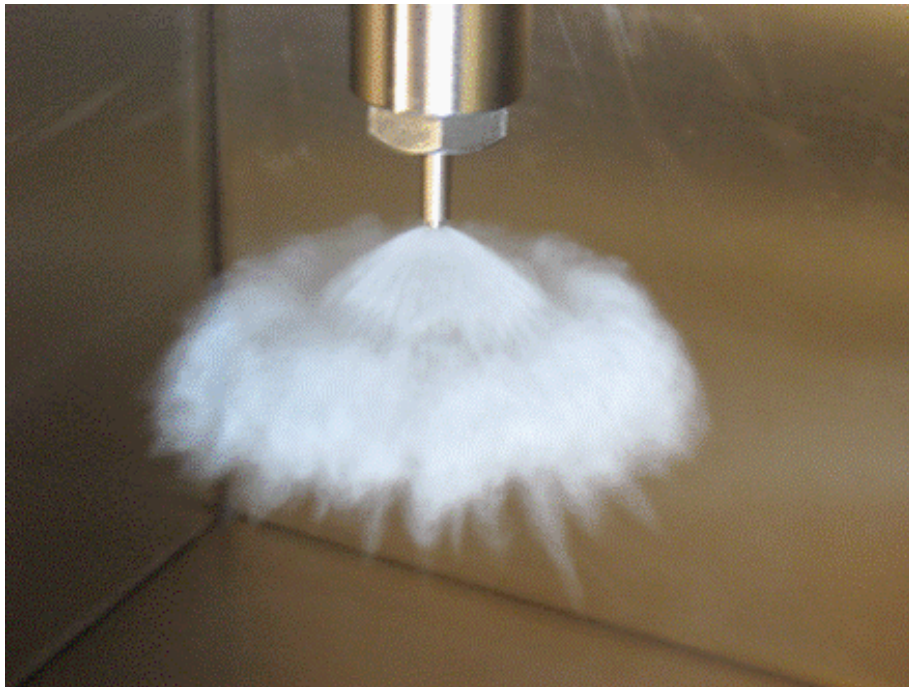
First phase injection with conical spray and narrow spray angle produced by MVCO Nozzle
