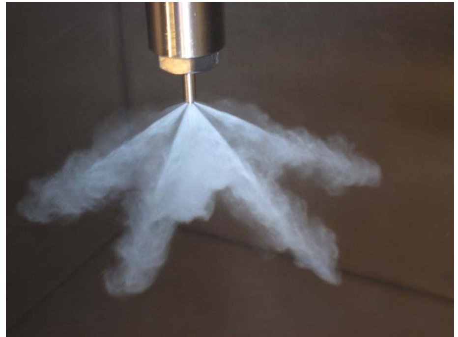
Second phase injection with multi-jet spray and wide spray angle produced by MVCO Nozzle
