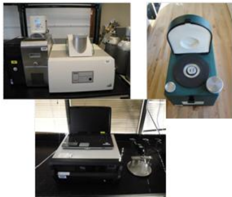
Figure II - 120: Thin film thermal conductivity meter, coin cell calorimeter, and bulk thermal conductivity meter (clockwise from upper left)
