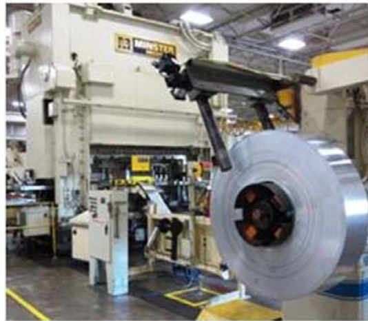
Figure II - 86: HTTP LLC, H&T, Trans-Matic Equipment – Battery Can Stamping Press.
