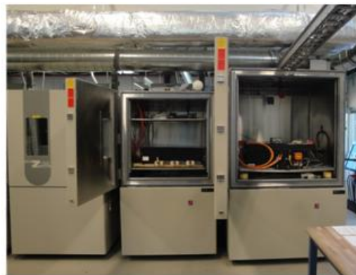
Figure II - 118: TTF Laboratory Environmental Chambers (3/5) with JCS and A123Systems PHEV battery packs under test.
