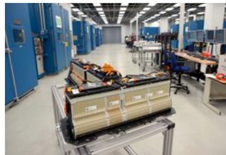
Figure II - 48: 2011 Chevrolet Volt Battery in the GM Battery Systems Lab in Warren, MI.
