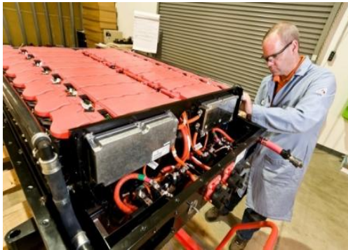
Figure II - 8: Complete battery packs and systems are assembled domestically prior to being sent to the customer.
