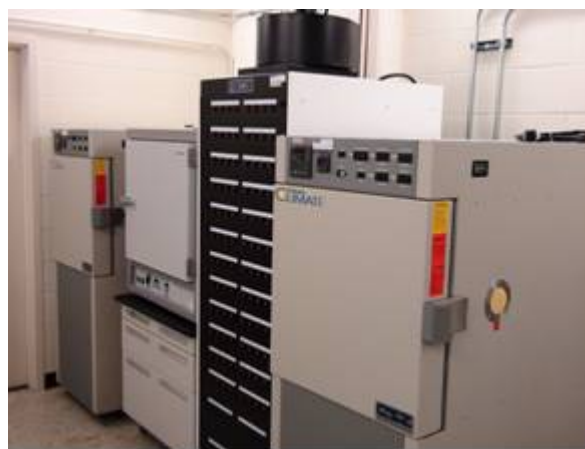
Figure II - 94: Maccor Series 4000 Automated Test System for testing and formation of prototype cells with environmental chambers and ovens.
