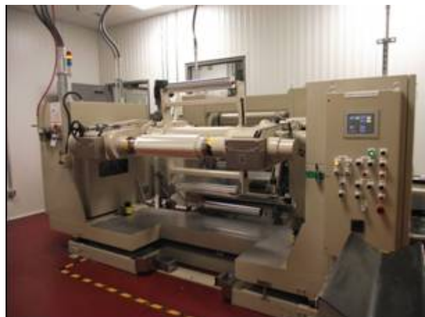
Figure II - 39: EnerDel Lithium-ion Cell Production and Battery Pack Assembly – Unwinder Anode Coater – Hague Rd.
