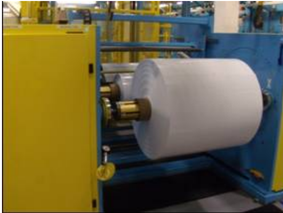
Figure II - 51: Fully formed flat sheet membrane from new equipment (Phase 1 Project in Charlotte, N.C.)
