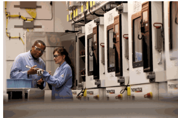
Figure II - 5: Johnson Controls' facilities include the equipment necessary to perform all relevant battery and cell tests, including cycle testing in controlled temperature environments.
