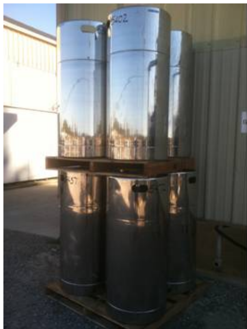
Figure II - 69: Several examples of the 400 215-L Electrolytes shipping vessels purchased in 2010.
