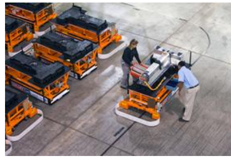
Figure II - 46: Battery Pack Assembly on Automated Guided Carts.
