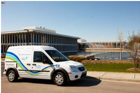
Figure II - 9: The Ford Transit Connect Electric features a 28 kWh Li-ion pack that was built in our Michigan plant.
