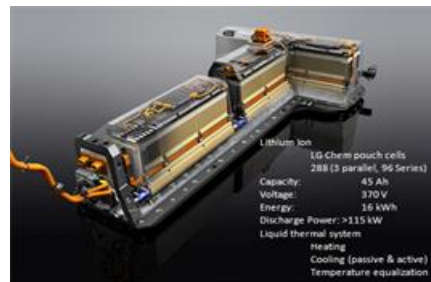
Figure II - 47: 2011 Chevrolet Volt Battery & Specifications.
