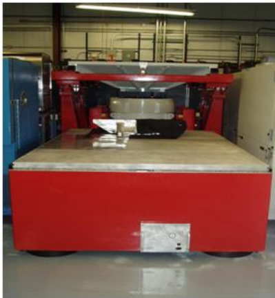
Figure II - 114: Vibration testing system for full size vehicle battery pack testing received in FY 2011.
