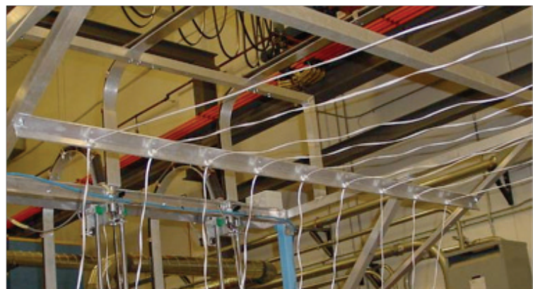
Figure 6. Fiber guides utilized to provide spacing and to mitigate tangling with 9 tow deposition.
