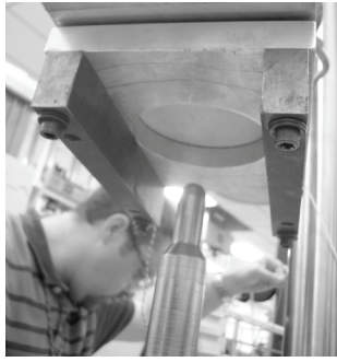
Figure 10. Multi-Axial Test Setup with Impactor (visible at the bottom of the image and specimen in the circular opening of the fixture)
