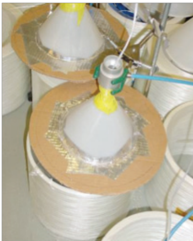
Figure 5. Air braking mechanism to mitigate fiber inertia problems.
