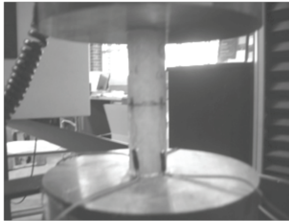
Figure 5. Experimental setup for filament wound crush tube testing.
