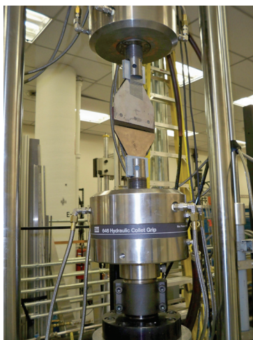
Figure 7. Torsion test of composite-to-steel weld bonded coupon in MTS Axial-Torsional test machine.
