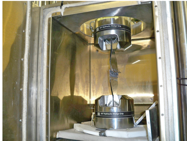
Figure 2. Super lap shear weld bonded specimen installed in ORNL mechanical test machine and oven.
