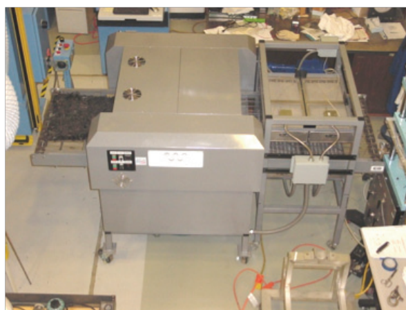
Figure 9. Combination IR and convection oven. (IR section surrounds conveyor entrance at right.)
