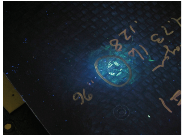
Figure 22. Impact site of 96-inch height ball drop, under UV light
