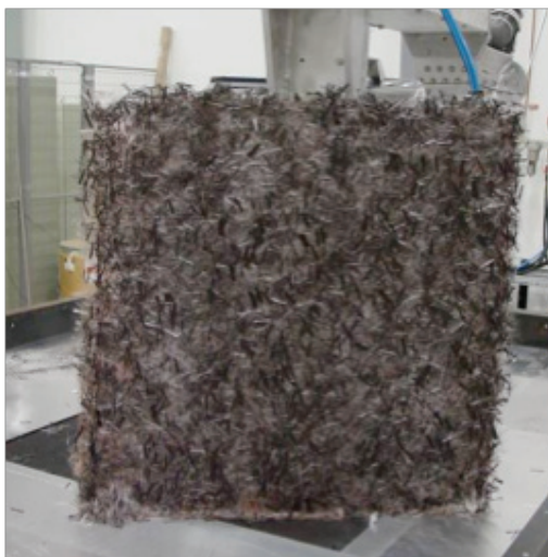
Figure 8. Hybrid carbon, glass, and polypropylene preform manufactured with upgraded chopper.
