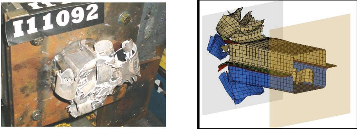
**Figure 4.** Deformed shape of sheet AZ31 double top hat beam after the high speed sled axial crush test, (a) physical test, (b) FEA prediction.
