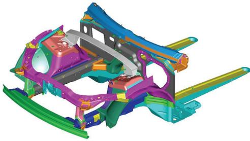
Figure 1. Unibody (BFI) steel front-end baseline structure for the donor vehicle.
