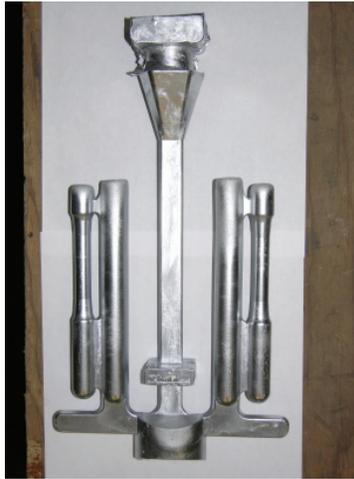
Figure 2. Cast of A356 aluminum alloy with larger mold
