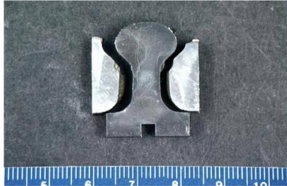
**Figure 2.** Sectioned bulkhead showing absence of interface bond between iron insert and magnesium bulkhead for DTS engine.
