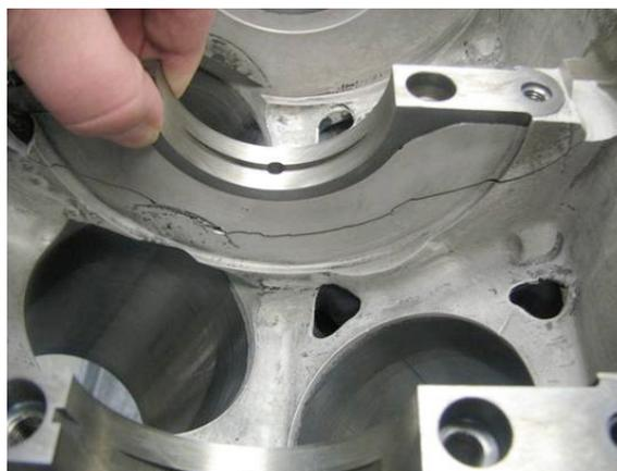
[Figure 1](#). Fracture of DTS engine bulkhead 3.
