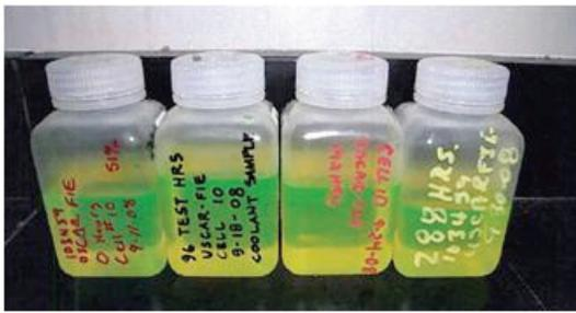
Figure 5. Coolant specimens taken from the engine during coolant corrosion testing.
