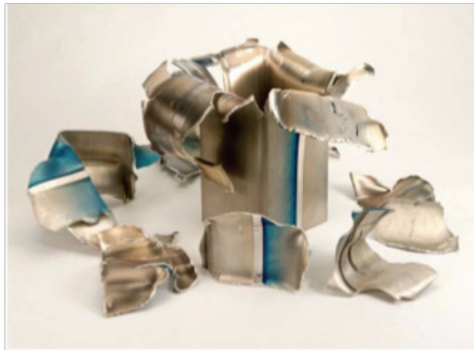
Figure 1. Mg Extrusion Exhibiting Low Ductility Failure
