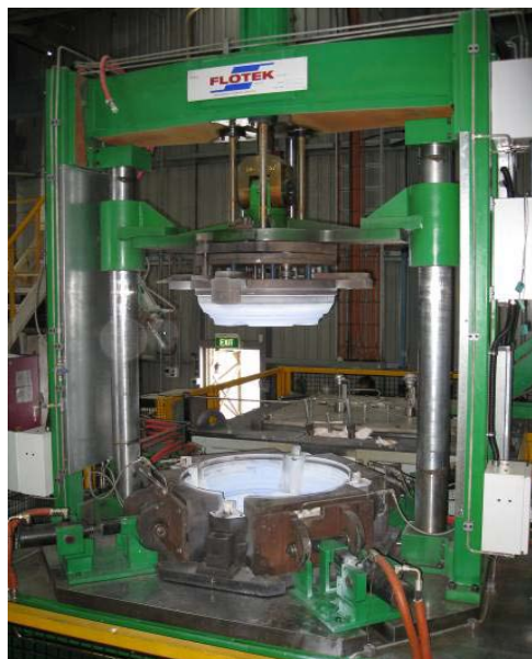
Figure 5. T-Mag casting cell.
