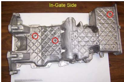
Figure 9. Structural oil pan showing locations of excised specimens.
