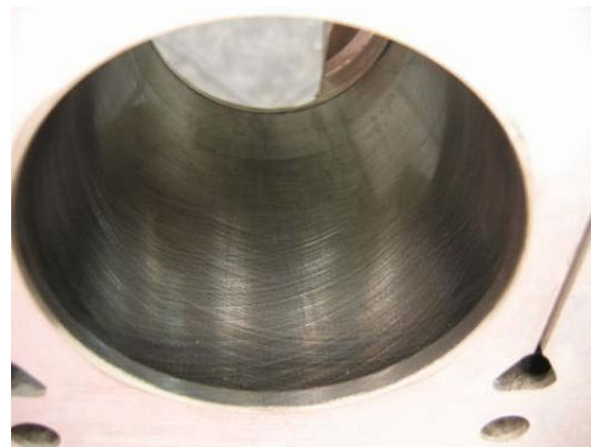
Figure 7. Cylinder bore at end of cold scuff test. Honing marks are evident.
