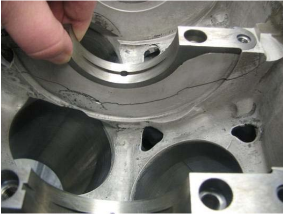
Figure 8. Fracture of DTS engine bulkhead 3.
