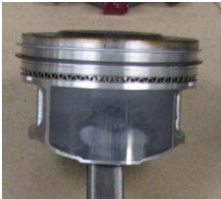
Figure 6. Post-hot scuff tested piston showing acceptable wear of the piston skirt coating.
